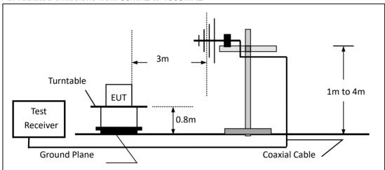
(c) For radiated emissions above 1000MHz
