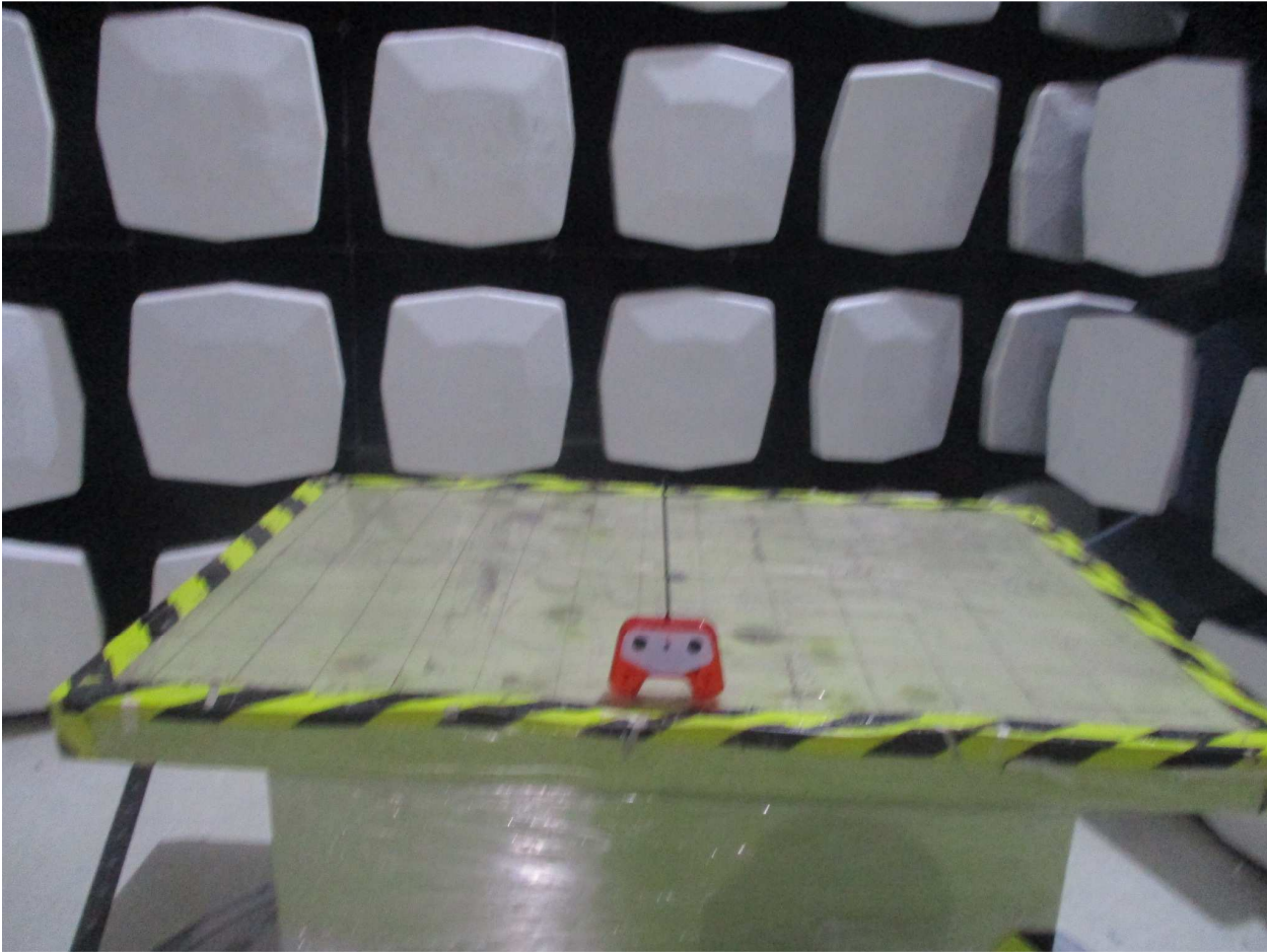
(EUT was placed in the center of the turntable)
