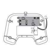
Insert the Circuit Board into the back side
