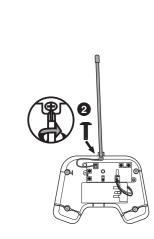
Attach the Antenna to the Rear Body.
