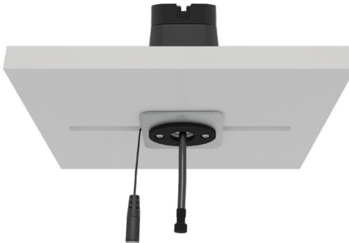
Insert the sensor cable into the pedestal and out through the center of the metal plate. The power cable should feed out the side of the mounting plate.
