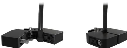
The VP-1644 cable stopper is installed behind the fixture. Open the stopper with a V-T41 security driver. Close the stopper in the groove at the end of the cable and tighten the screw again.
