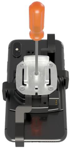
Place the device and bracket face down on a flat surface. This holds the arms in place while tightening the screw. Align the bracket to the center of the device. Tighten the screw on the back of the bracket assembly with the security driver.
