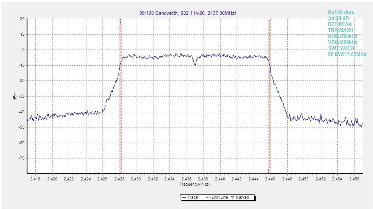
Fig.41 99% Occupied Bandwidth (802.11n-20MHz, Ch 6)
