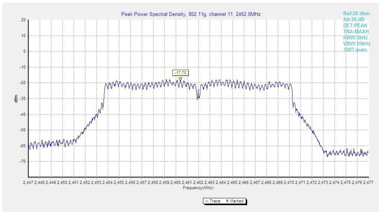
Fig.6 Power Spectral Density (802.11g, CH 11)
