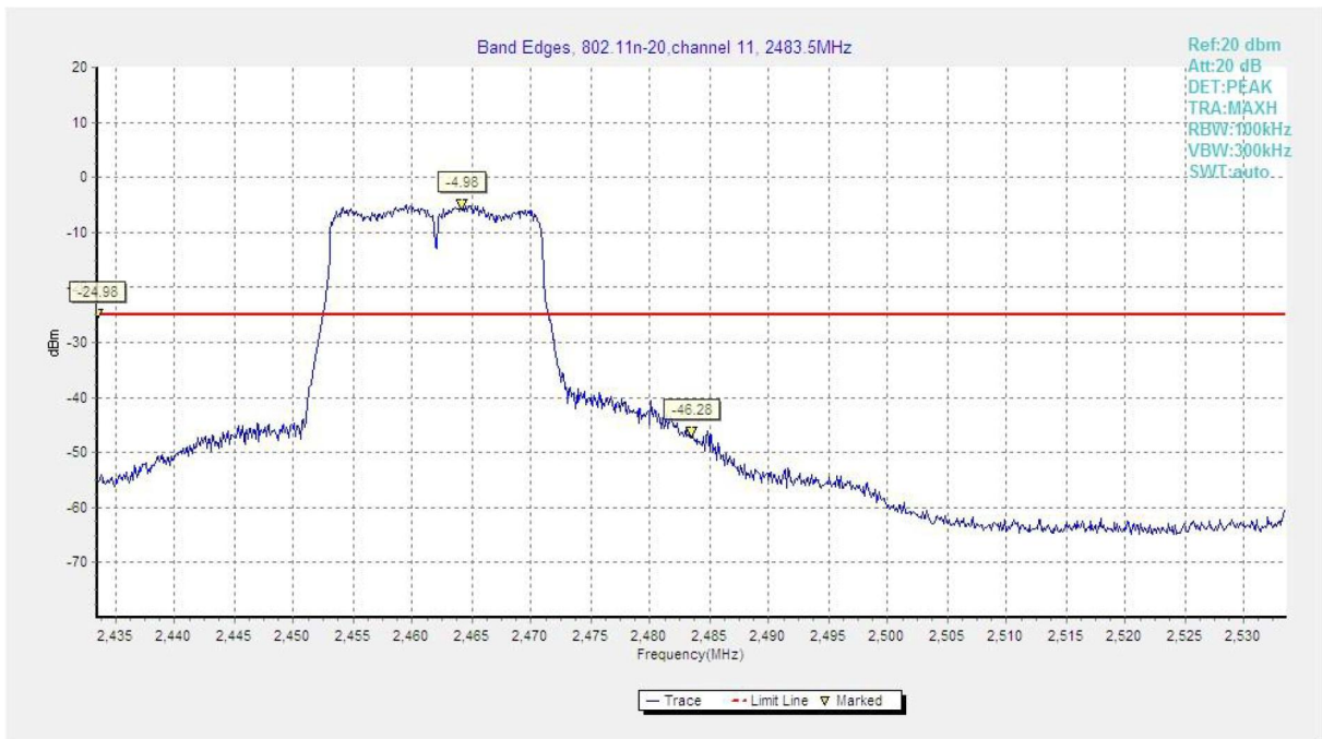
Fig.24 Band Edges (802.11n HT20, CH 11)
