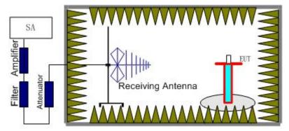
2. The EUT is then put into continuously transmitting mode at its maximum power level during the test. And the maximum value of the receiver should be recorded as (Pr). The placement of EUT and AE is shown in the figure below, what's more, The EUT was tested in two states, horizontal and vertical as show in the attachment.
