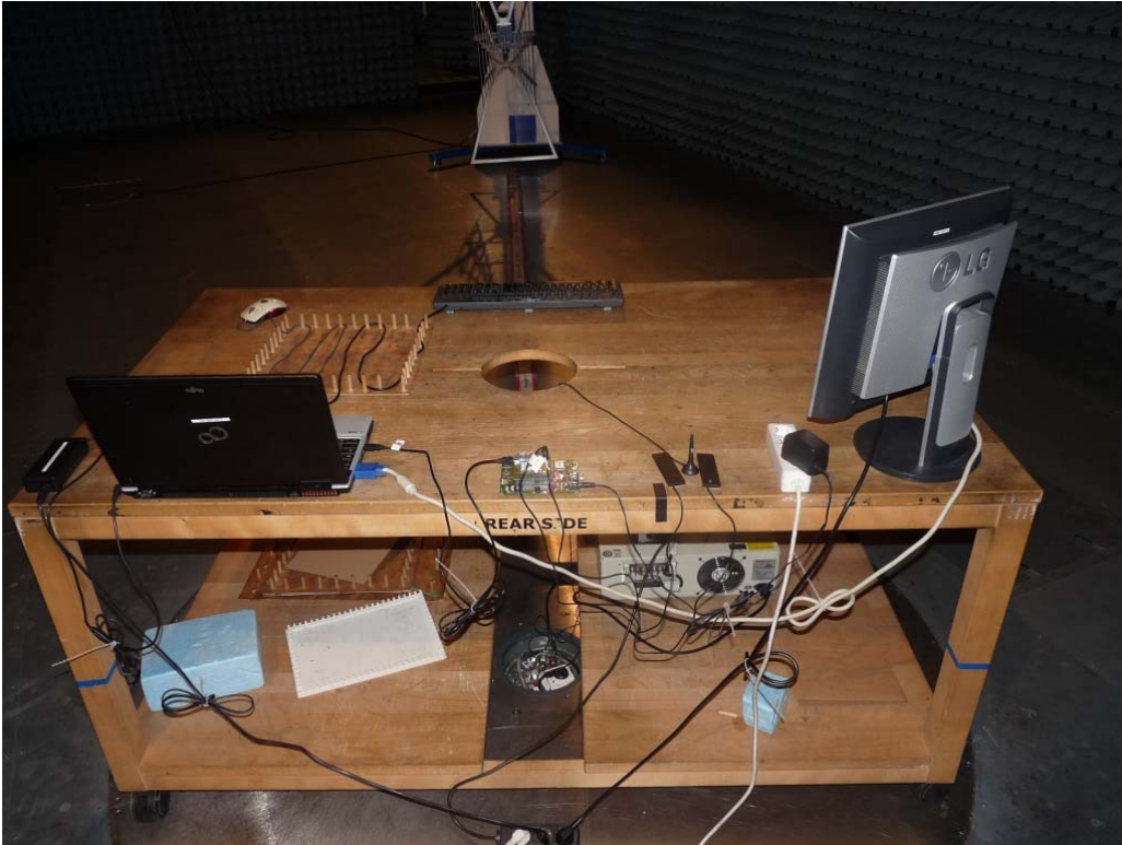
Photo 4: Test setup for radiated measurements (computer peripheral setup, EUT supplied by AC adapter, unintentional radiator §15)
