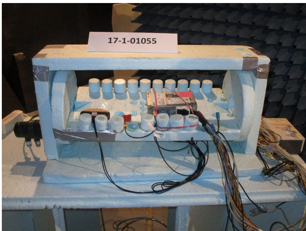
Test setup in semi anechoic room close up view EUT standing
