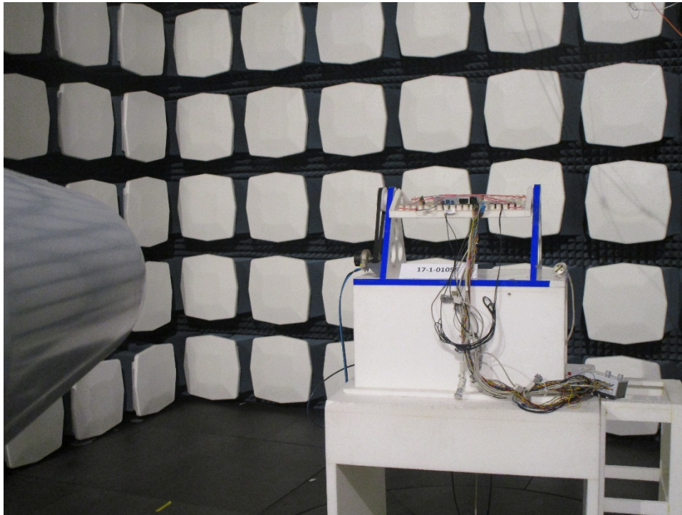
Setup in fully anechoic room long shot EUT laying
