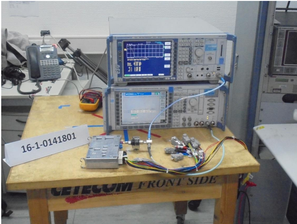
Photograph 7: Set-up for power measurements (Cellular power and CCDF)
