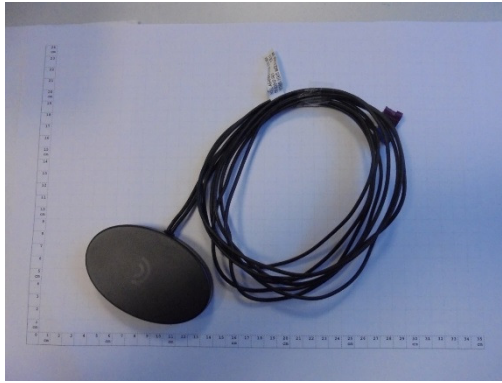
Photograph 7: Cellular/ GNSS antenna
