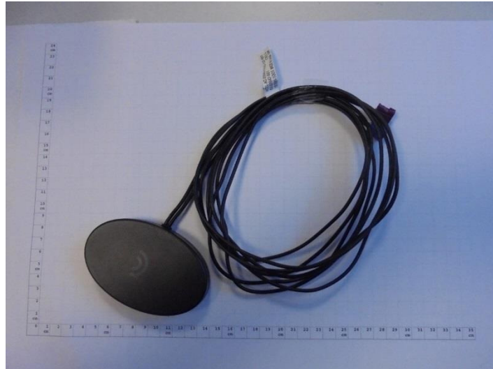
Photograph 7: Cellular/ GNSS antenna
