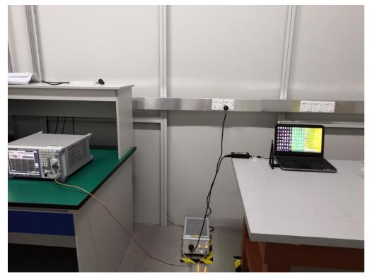
FCC RADIATED EMISSION TEST SETUP BELOW 1GHZ
