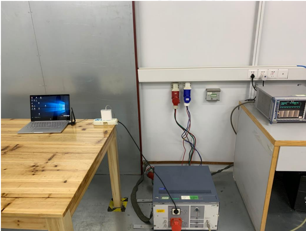
FCC RADIATED EMISSION TEST SETUP BELOW 1GHZ
