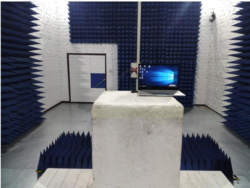
FCC RADIATED EMISSION TEST SETUP ABOVE 1GHZ
