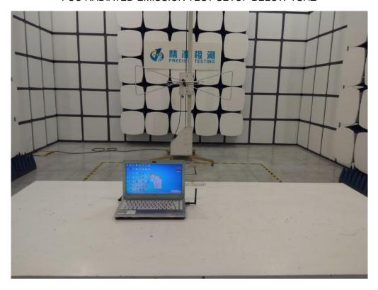
FCC RADIATED EMISSION TEST SETUP ABOVE 1GHZ
