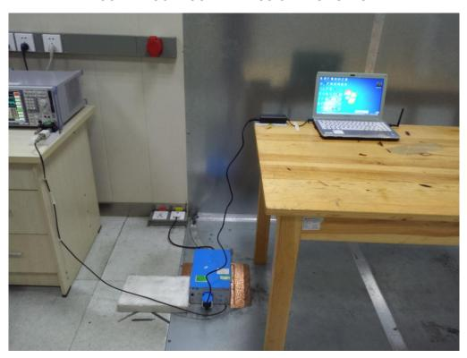
FCC RADIATED EMISSION TEST SETUP BELOW 1GHZ
