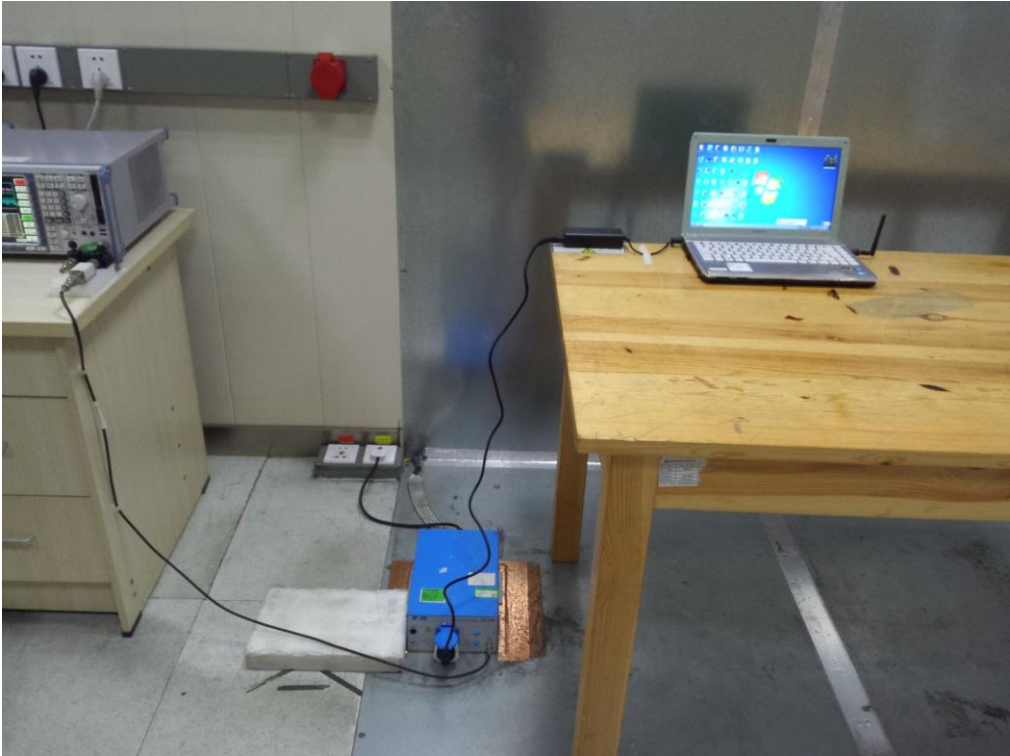
FCC RADIATED EMISSION TEST SETUP BELOW 1GHZ
