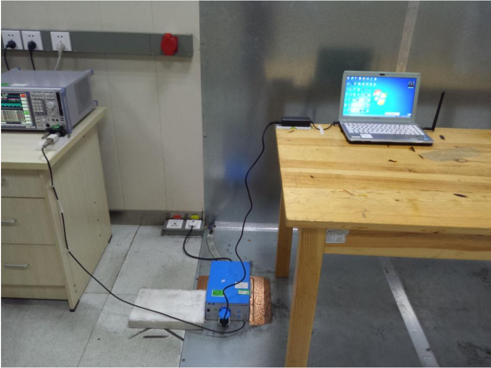
FCC RADIATED EMISSION TEST SETUP BELOW 1GHZ
