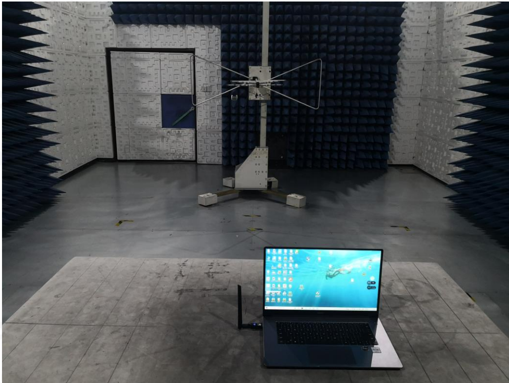
FCC RADIATED EMISSION TEST SETUP ABOVE 1GHZ
