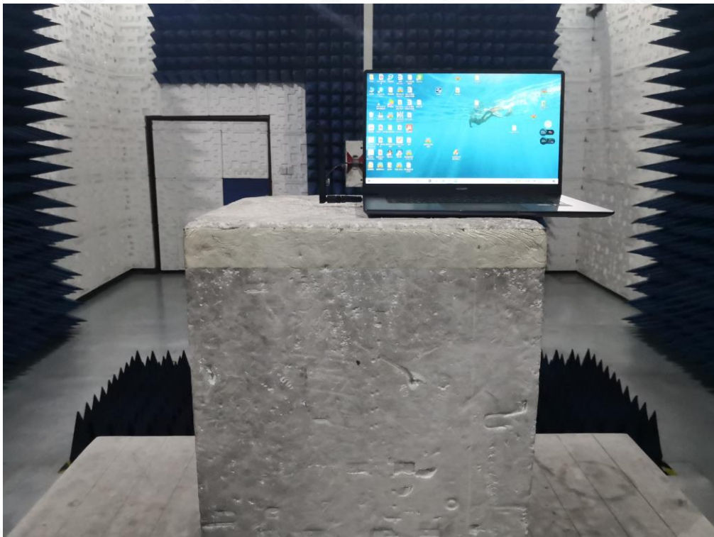
FCC RADIATED EMISSION TEST SETUP ABOVE 1GHZ
