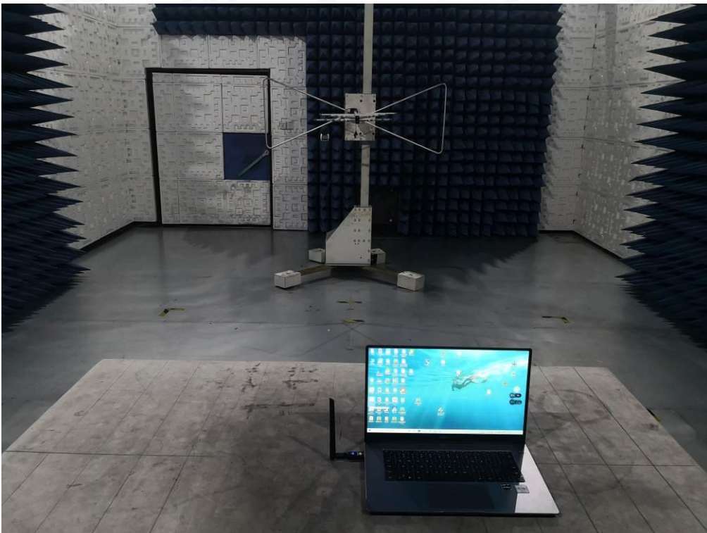
FCC RADIATED EMISSION TEST SETUP BELOW 1GHZ
