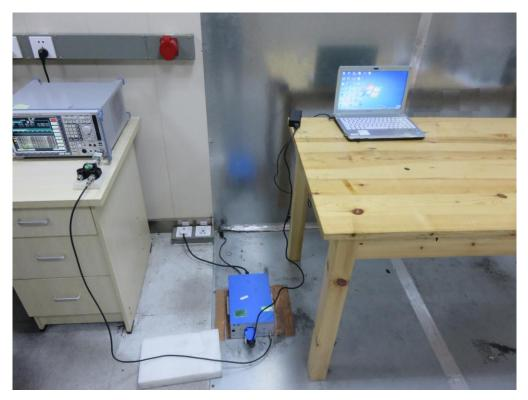
FCC RADIATED EMISSION TEST SETUP
