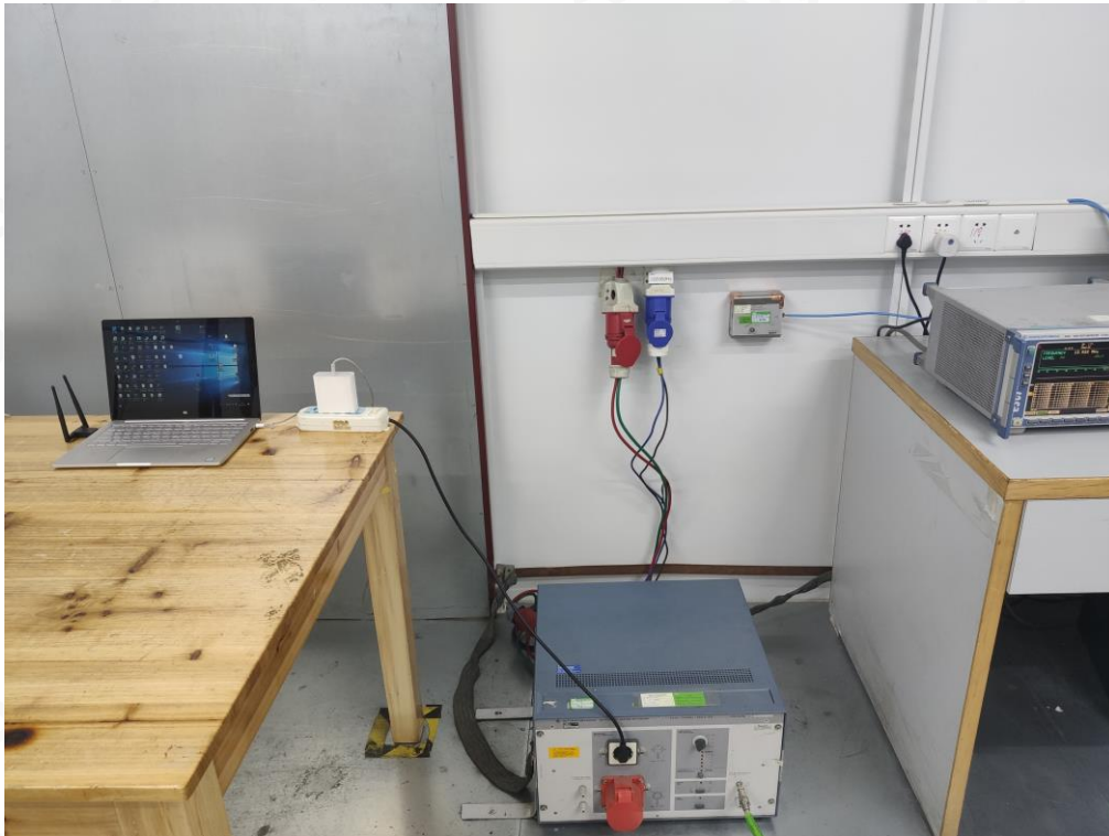
FCC RADIATED EMISSION TEST SETUP BELOW 1GHZ
