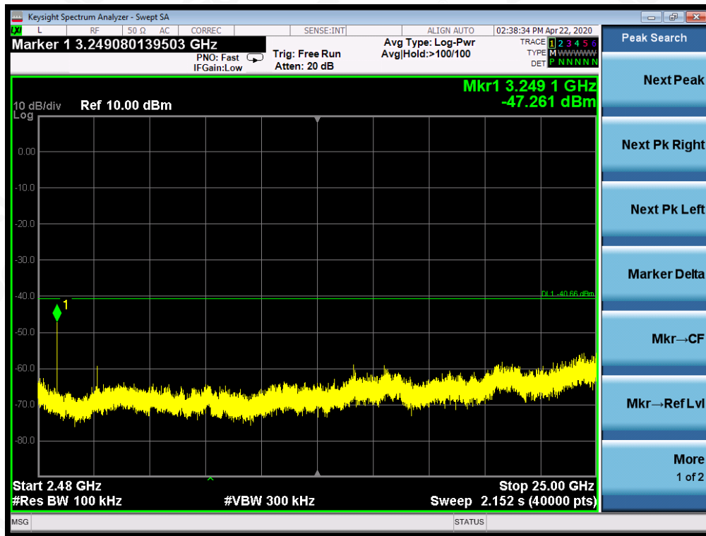
TEST PLOT OF OUT OF BAND EMISSIONS THE WORST CASE OF 802.11n40 FOR MODULATION IN HIGH CHANNEL
