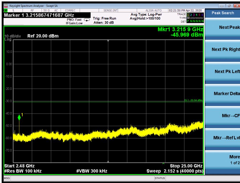
TEST PLOT OF OUT OF BAND EMISSIONS THE WORST CASE OF 802.11b FOR MODULATION IN MIDDLE CHANNEL
