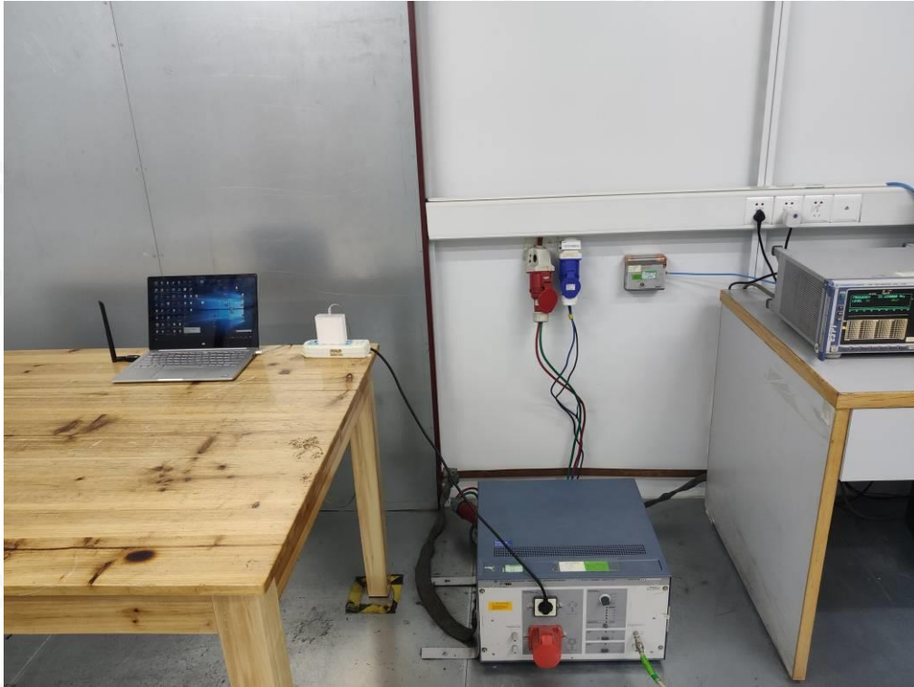
FCC RADIATED EMISSION TEST SETUP BELOW 1GHZ
