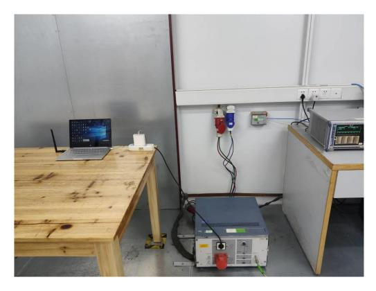
FCC RADIATED EMISSION TEST SETUP BELOW 1GHZ
