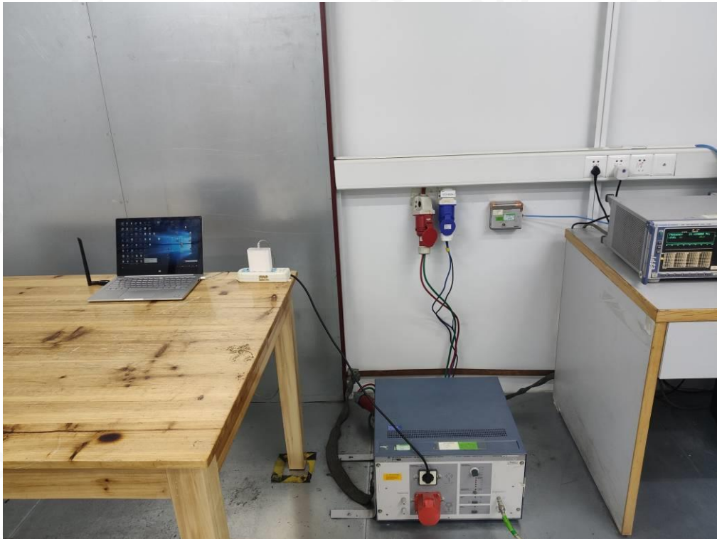
FCC RADIATED EMISSION TEST SETUP BELOW 1GHZ
