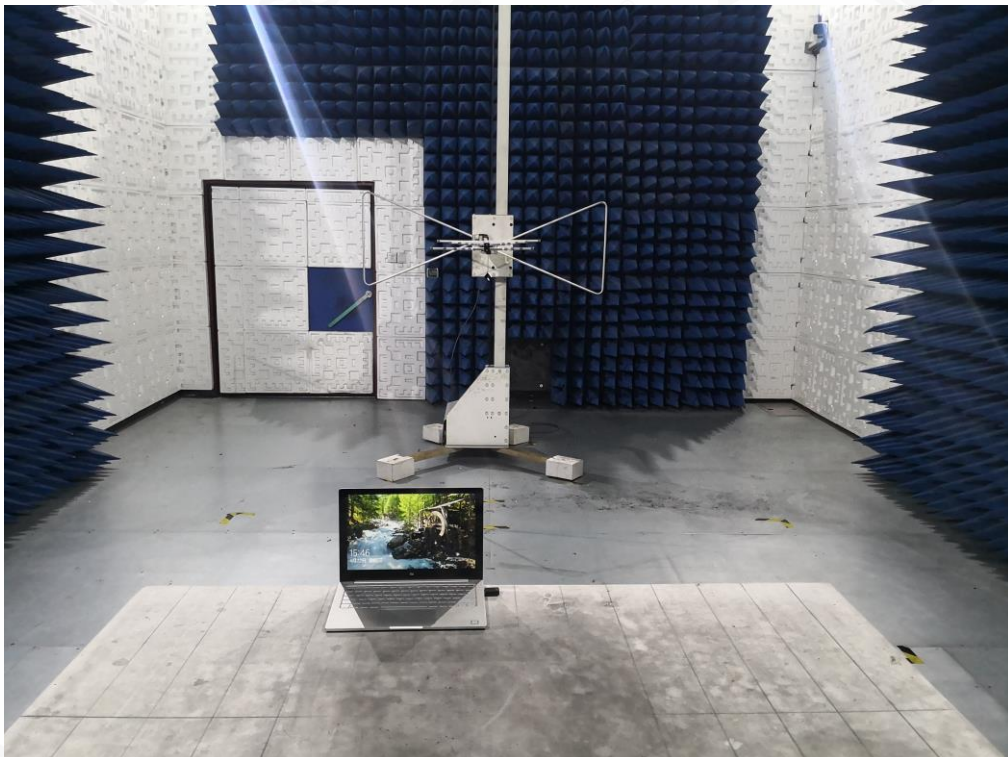
FCC RADIATED EMISSION TEST SETUP BELOW 1GHZ
