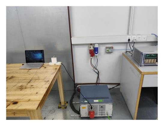
FCC RADIATED EMISSION TEST SETUP BELOW 1GHZ
