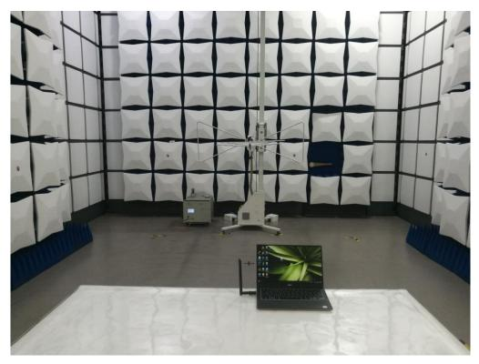
FCC RADIATED EMISSION TEST SETUP ABOVE 1GHZ
