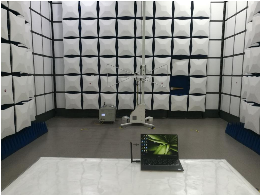
FCC RADIATED EMISSION TEST SETUP BELOW 1GHZ
