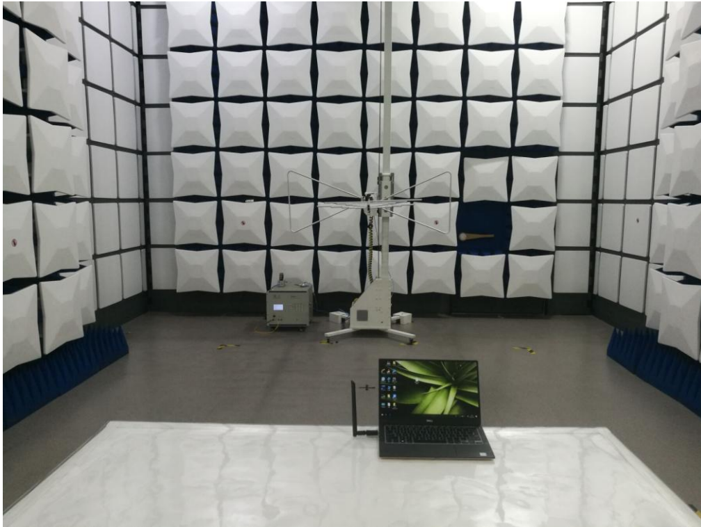
FCC RADIATED EMISSION TEST SETUP ABOVE 1GHZ
