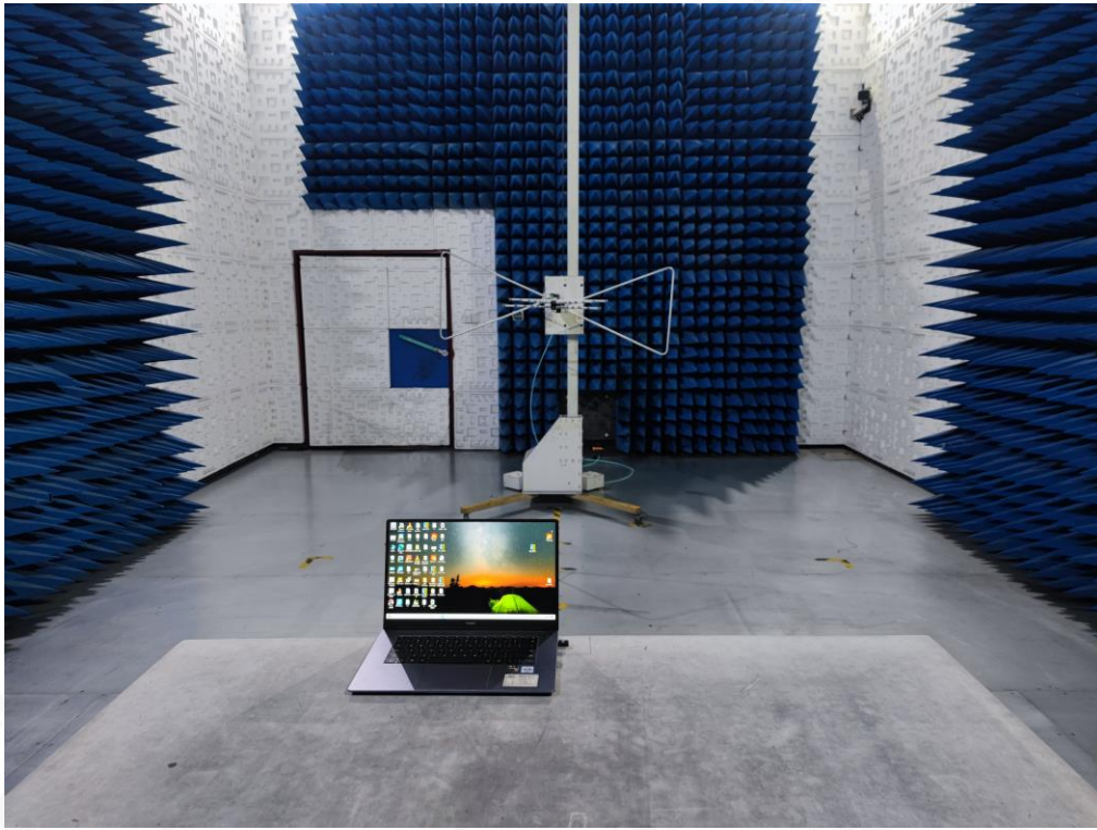
RADIATED EMISSION TEST SETUP ABOVE 1GHZ
