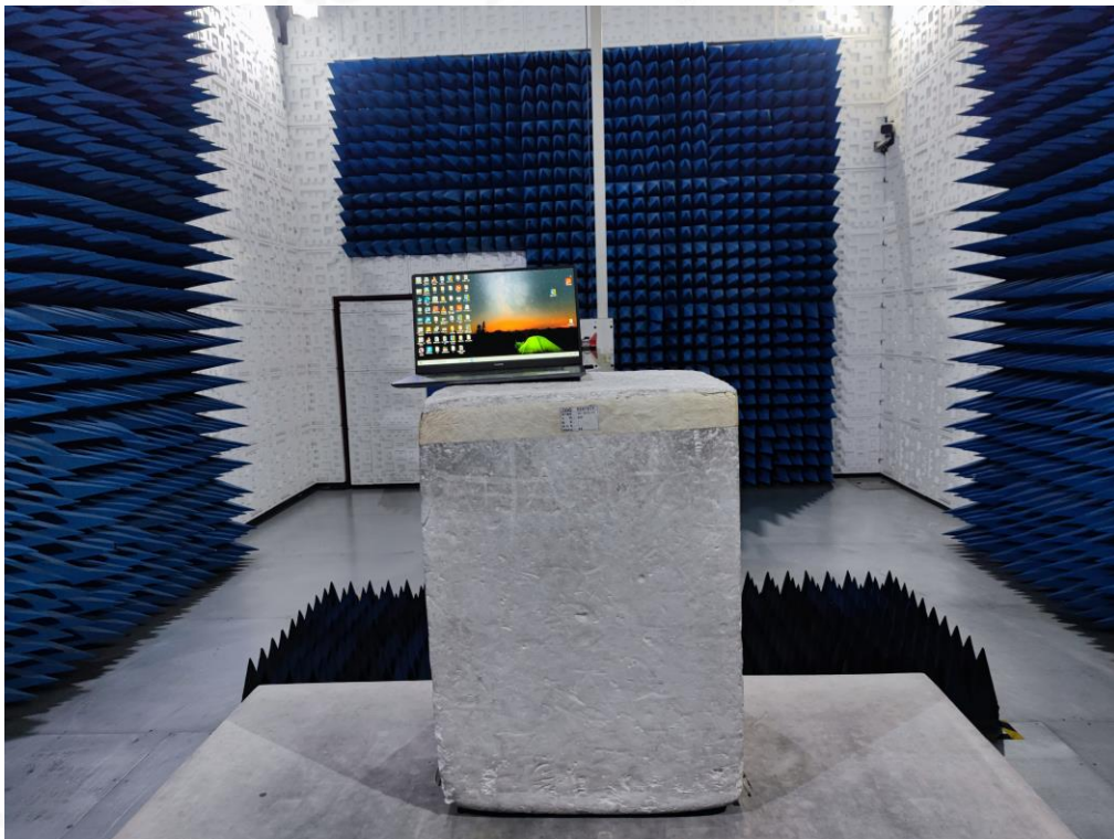
RADIATED EMISSION TEST SETUP ABOVE 1GHZ
