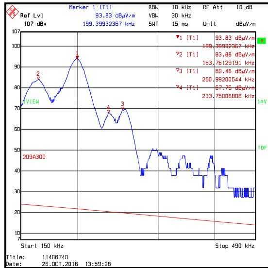
150 kHz to 490 kHz / average detector / EUT operating / measured at 3 metres on an open field test site
