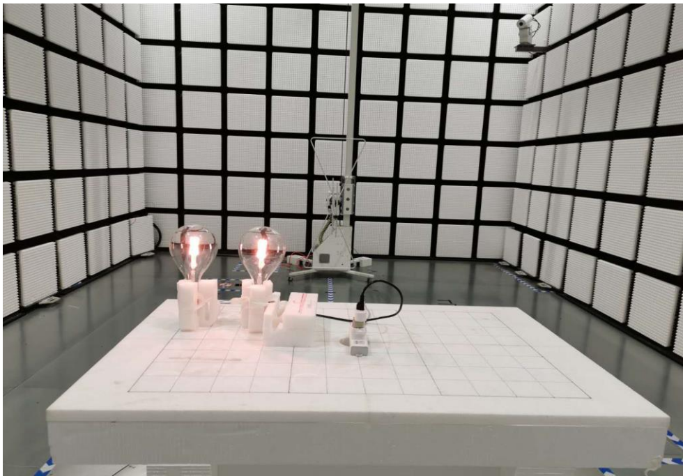
Fig.2 Radiated emission setup photo(30MHz-1GHz)
