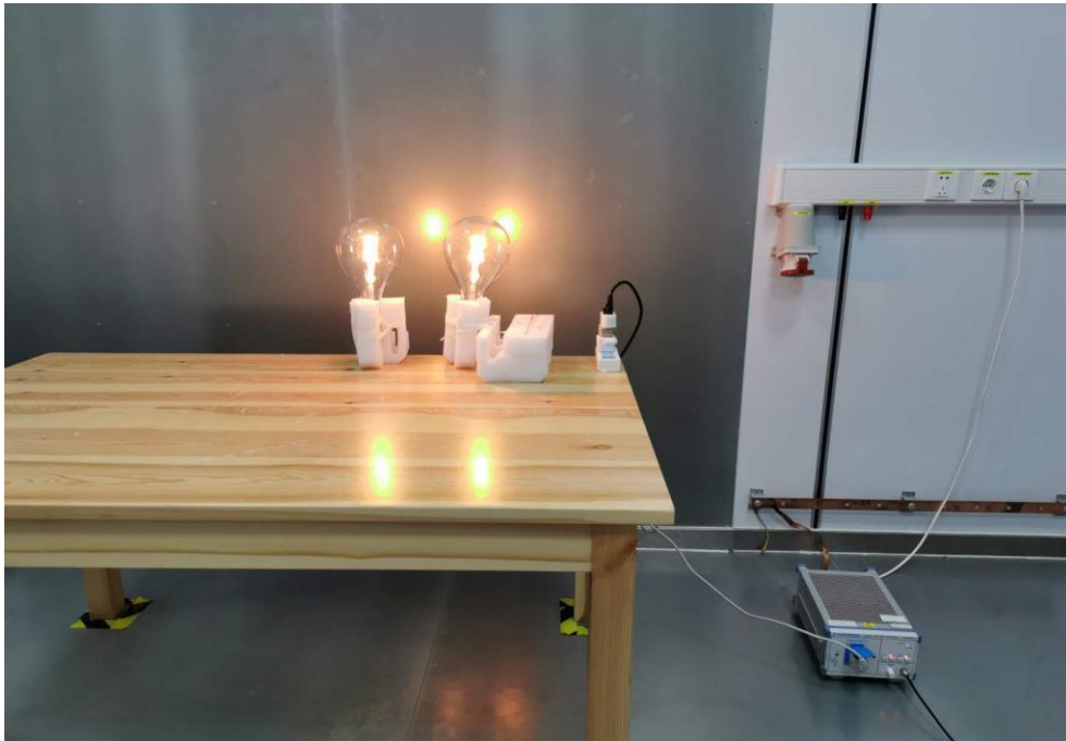
Fig.4 Power line conducted emission setup photo
