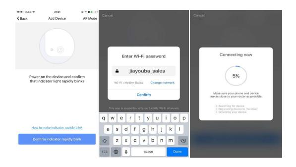
Step 4: Enter the device page, then complete the configuration
