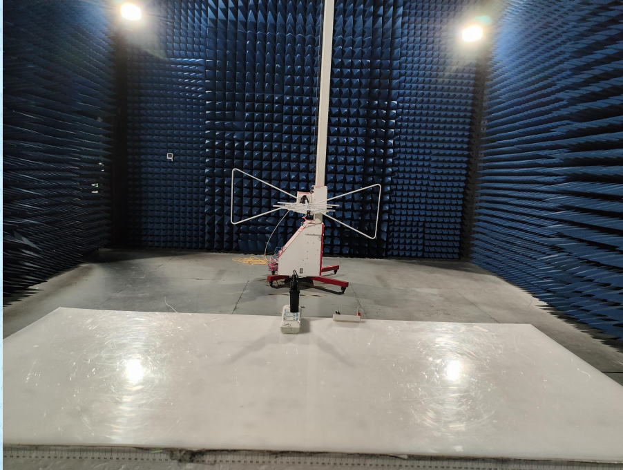
Radiated Emission Above 1GHz Test Setup
