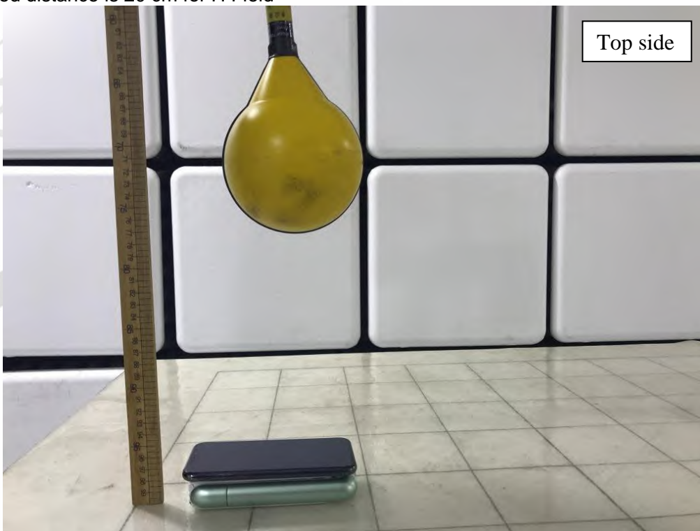
Measured distance is 20 cm for H Field
