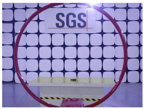
1.3 Radiated Emissions (30MHz-1GHz) Test Setup
