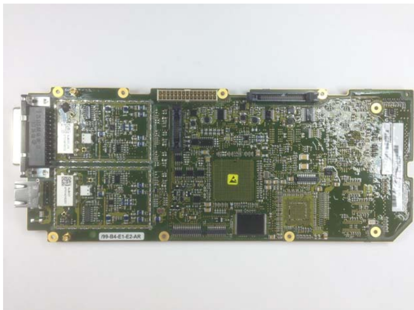
DPIO board Bottom Side without shield covers
