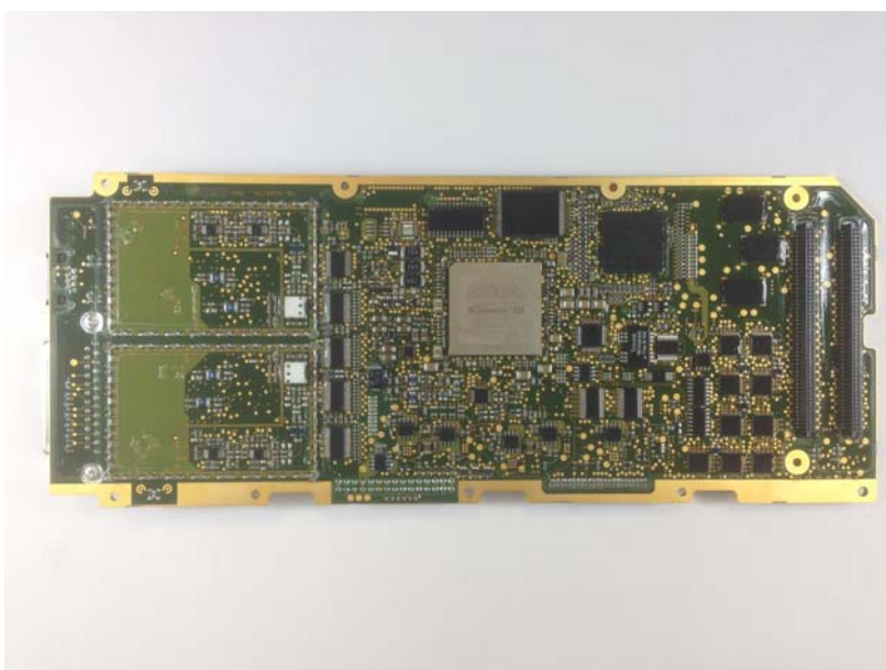
DPIO board Bottom Side without shield covers
