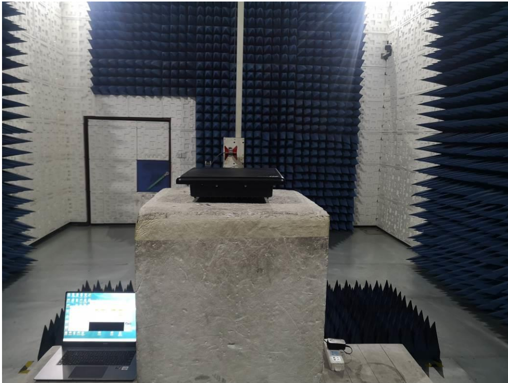
FCC RADIATED EMISSION TEST SETUP-ABOVE 1GHz
