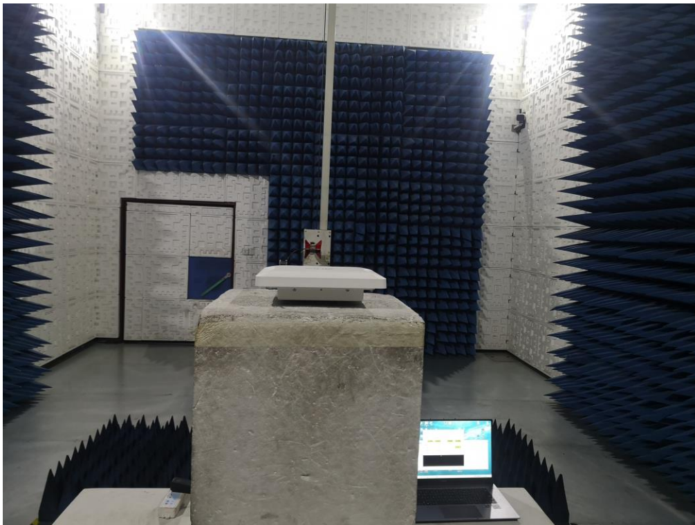
FCC RADIATED EMISSION TEST SETUP-ABOVE 1GHz
