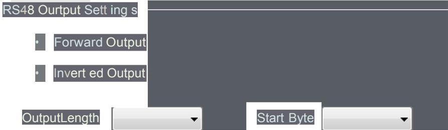
The RS485 Output Settings consist of Forward Output and Inverted Output. Click Forward Output to read the card number in the partition in the progressive order, and click Inverted Output to read out the card number in the partition in the reverse order.
