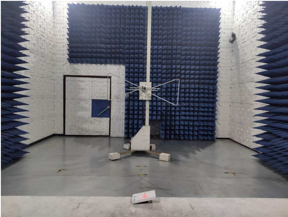
RADIATED EMISSION TEST SETUP BELOW 1GHz
