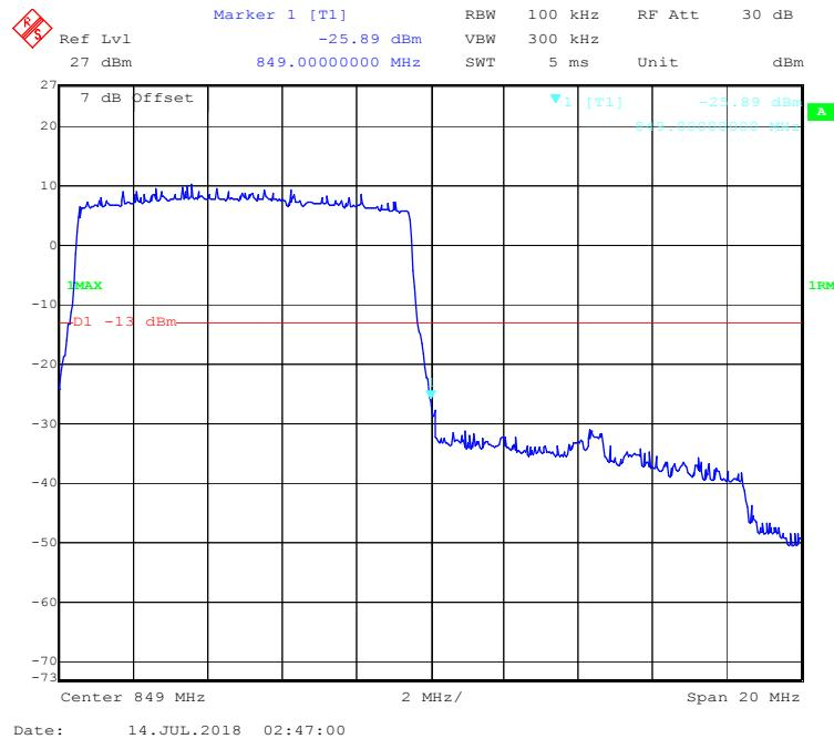
**16-QAM (1.4 MHz, FULL RB) - Left Band Edge**
