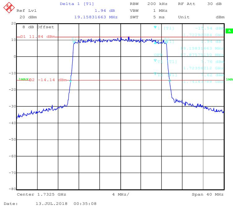
**16-QAM (1.4 MHz) - 99% Occupied & 26 dB Emissions Bandwidth, Middle channel**
