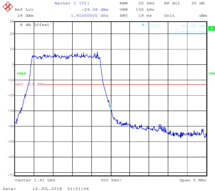
**16-QAM (3.0 MHz, FULL RB) - Left Band Edge**
