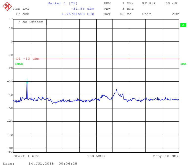
**LTE Band 17:****30 MHz - 1 GHz (5.0 MHz, Middle Channel)**
