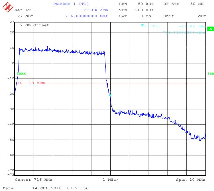
**16-QAM (10.0 MHz, FULL RB) - Left Band Edge**
