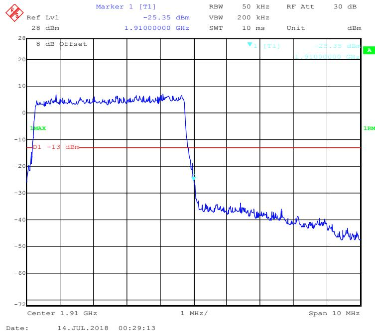
**QPSK (10.0 MHz, FULL RB) - Left Band Edge**
