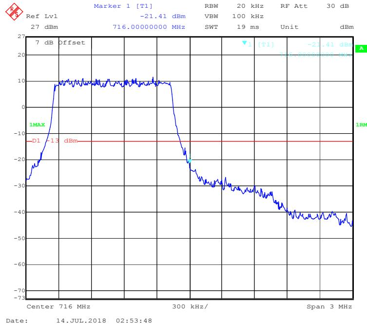
**QPSK (3.0 MHz, FULL RB) - Left Band Edge**
