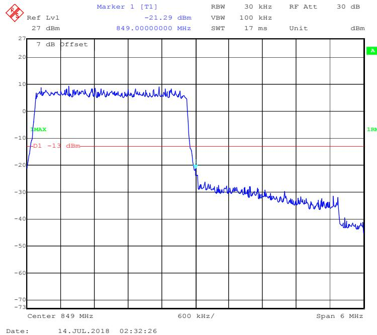
**QPSK (5.0 MHz, FULL RB) - Left Band Edge**
