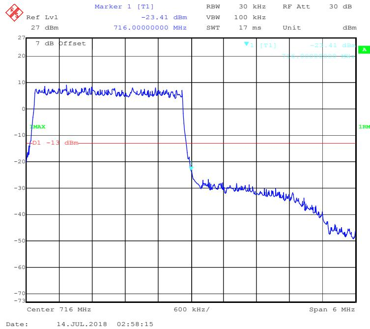
**QPSK (5.0 MHz, FULL RB) - Left Band Edge**
