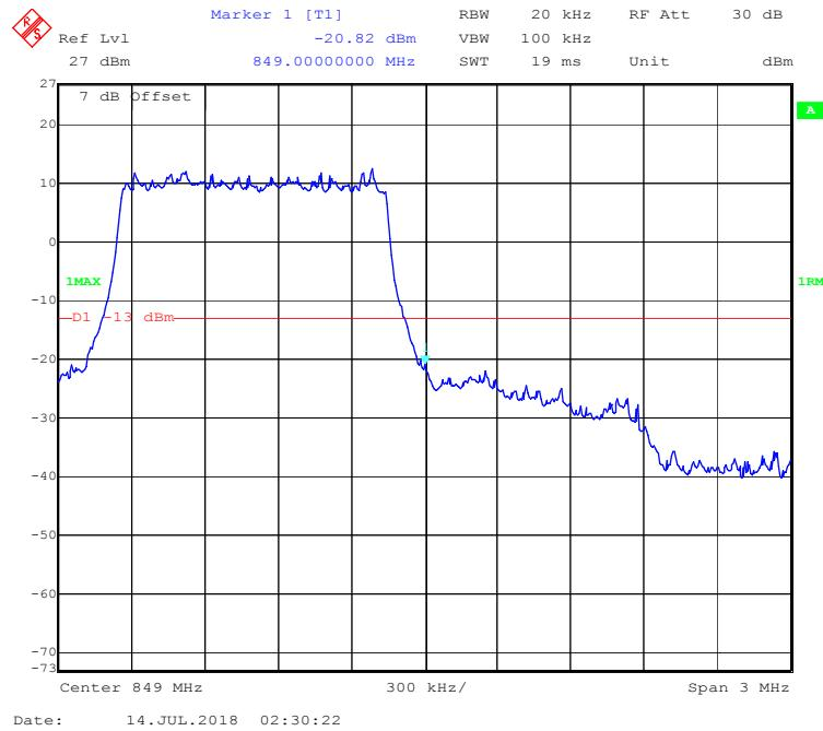
**16-QAM (3.0 MHz, FULL RB) - Left Band Edge**
