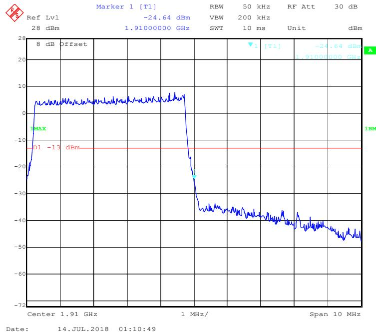
**16-QAM (10.0 MHz, FULL RB) - Left Band Edge**
