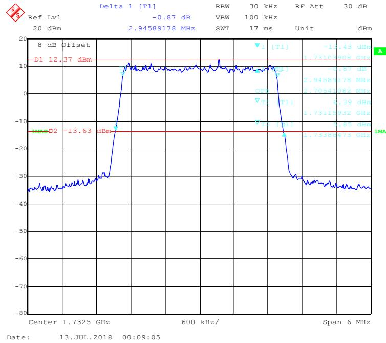
**16-QAM (5.0 MHz) - 99% Occupied & 26 dB Emissions Bandwidth, Middle channel**
