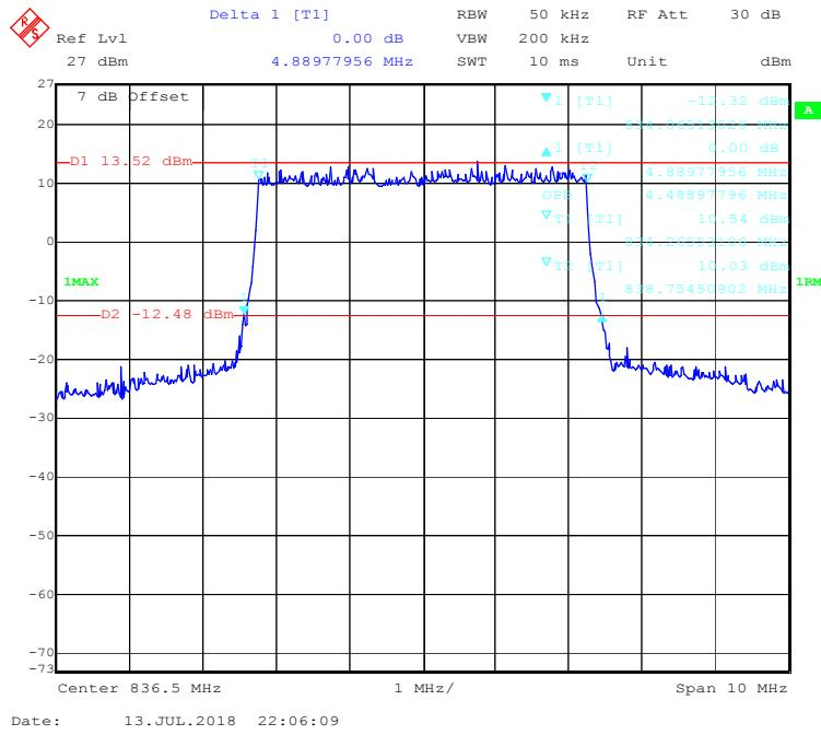
**QPSK (10.0 MHz) - 99% Occupied & 26 dB Emissions Bandwidth, Middle channel**
