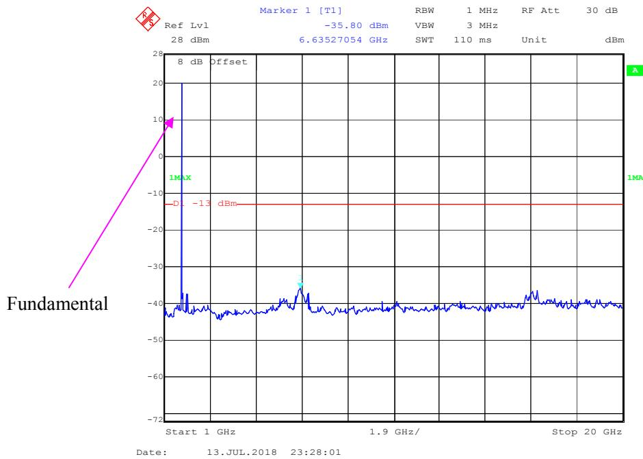
**30 MHz - 1 GHz (10.0 MHz, Middle Channel)**
