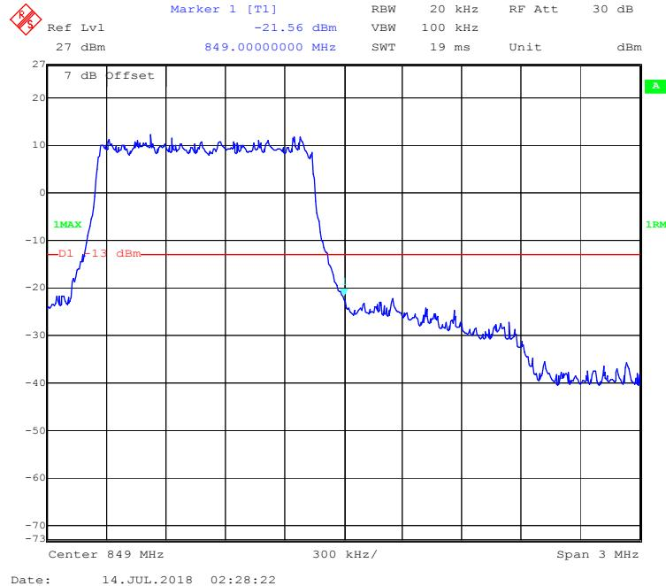
**QPSK (3.0 MHz, FULL RB) - Left Band Edge**
