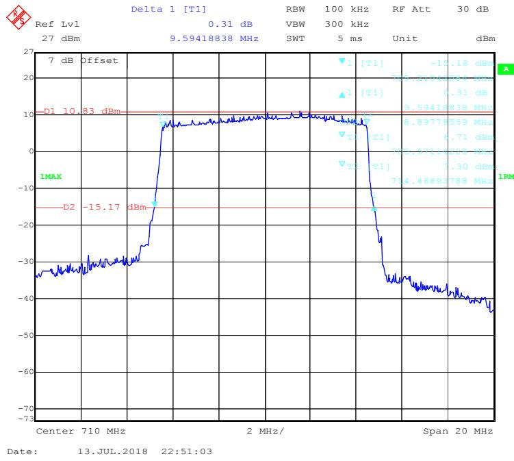
**FCC § 2.1051; § 22.917 (a); § 24.238 (a); §27.53 (h) (m) - SPURIOUS EMISSIONS AT ANTENNA TERMINALS****Applicable Standards**
