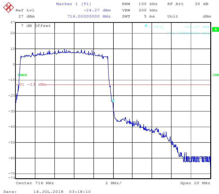
**16-QAM (5.0 MHz, FULL RB) - Left Band Edge**
