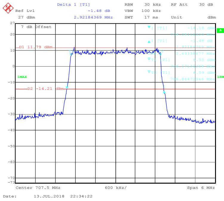
**16-QAM (5.0 MHz) -99% Occupied & 26 dB Emissions Bandwidth, Middle channel**
