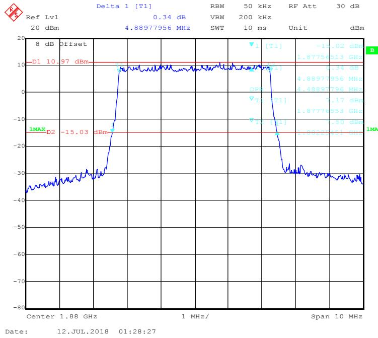
**16-QAM (10.0 MHz) - 99% Occupied & 26 dB Emissions Bandwidth, Middle channel**
