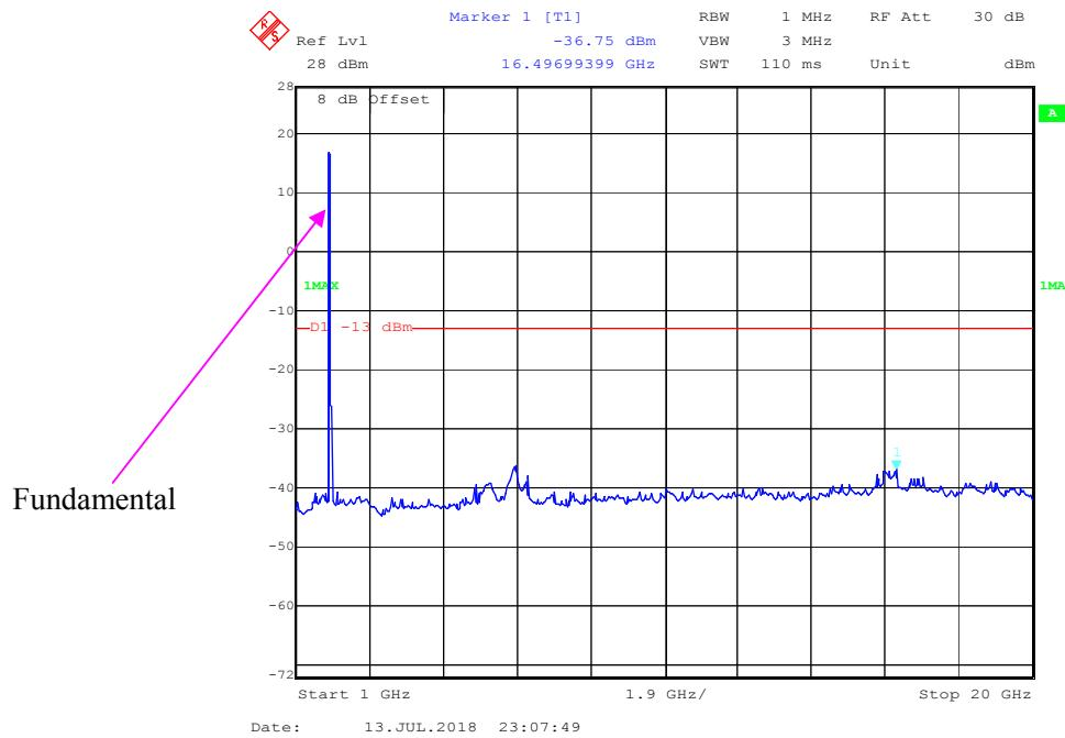
**30 MHz - 1 GHz (10.0 MHz, Middle Channel)**
