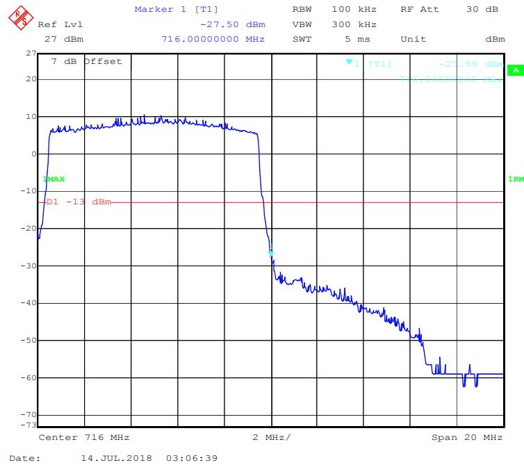
**LTE Band 17:****QPSK (5.0 MHz, FULL RB) - Left Band Edge**
