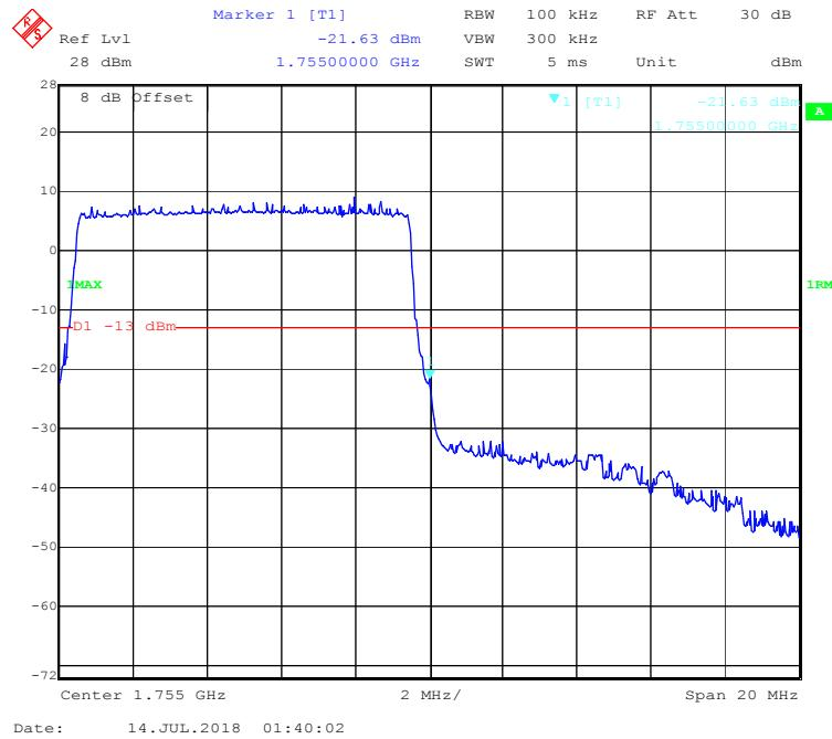
**16-QAM (15.0 MHz, FULL RB) - Left Band Edge**
