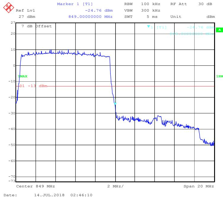
**LTE Band 12:****QPSK (1.4 MHz, FULL RB) - Left Band Edge**
