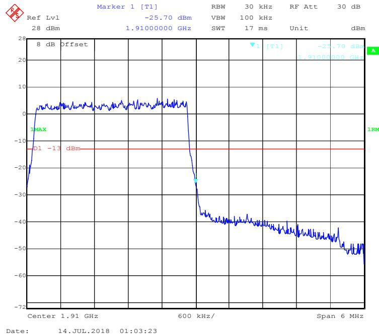
**16-QAM (5.0 MHz, FULL RB) - Left Band Edge**
