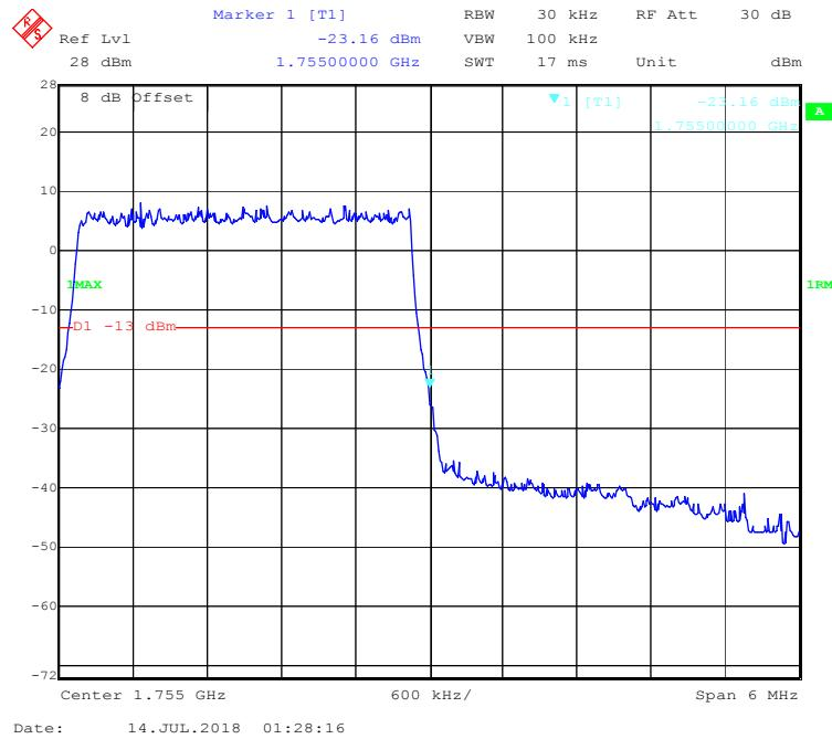
**16-QAM (5.0 MHz, FULL RB) - Left Band Edge**
