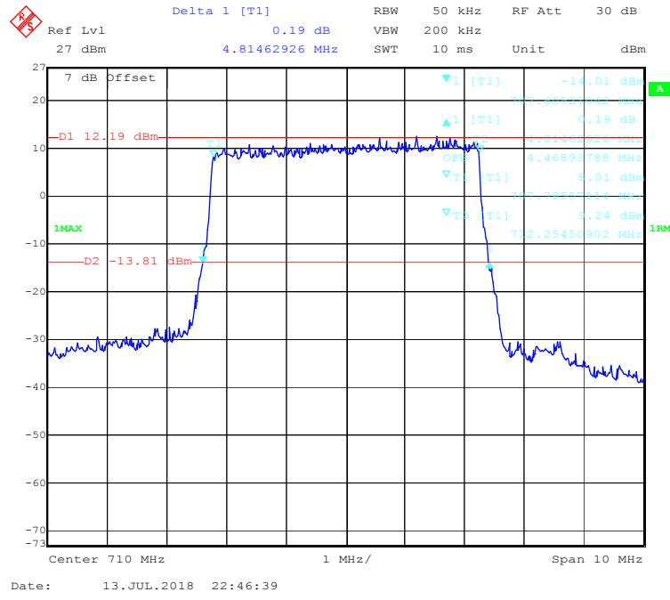
**QPSK (10.0 MHz) - 99% Occupied & 26 dB Emissions Bandwidth, Middle channel**
