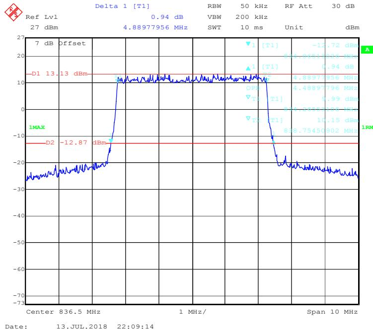
**16-QAM (10.0 MHz) - 99% Occupied & 26 dB Emissions Bandwidth, Middle channel**
