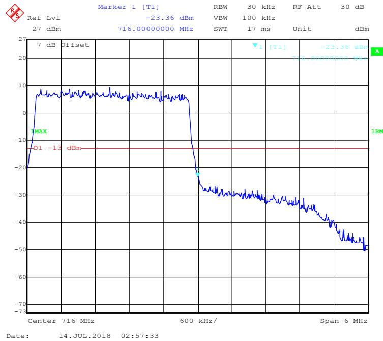
**16-QAM (5.0 MHz, FULL RB) - Left Band Edge**
