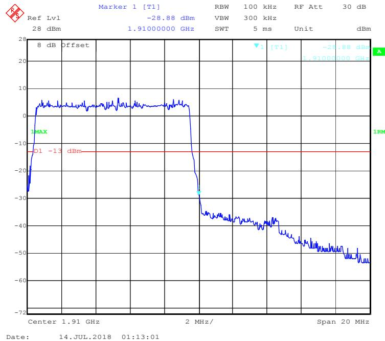
**16-QAM (15.0 MHz, FULL RB) - Left Band Edge**
