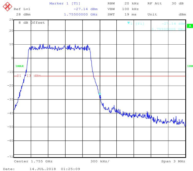
**16-QAM (3.0 MHz, FULL RB) - Left Band Edge**
