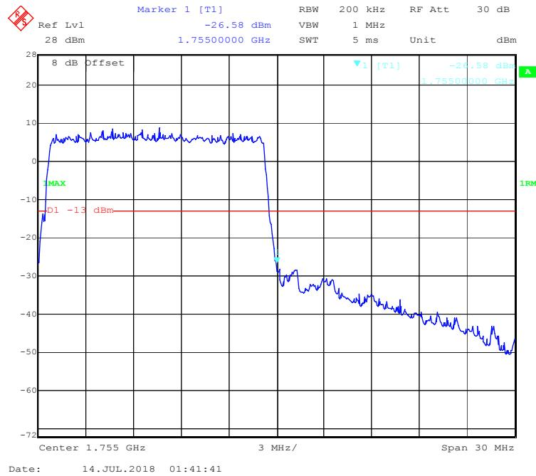
**16-QAM (20.0 MHz, FULL RB) - Left Band Edge**
