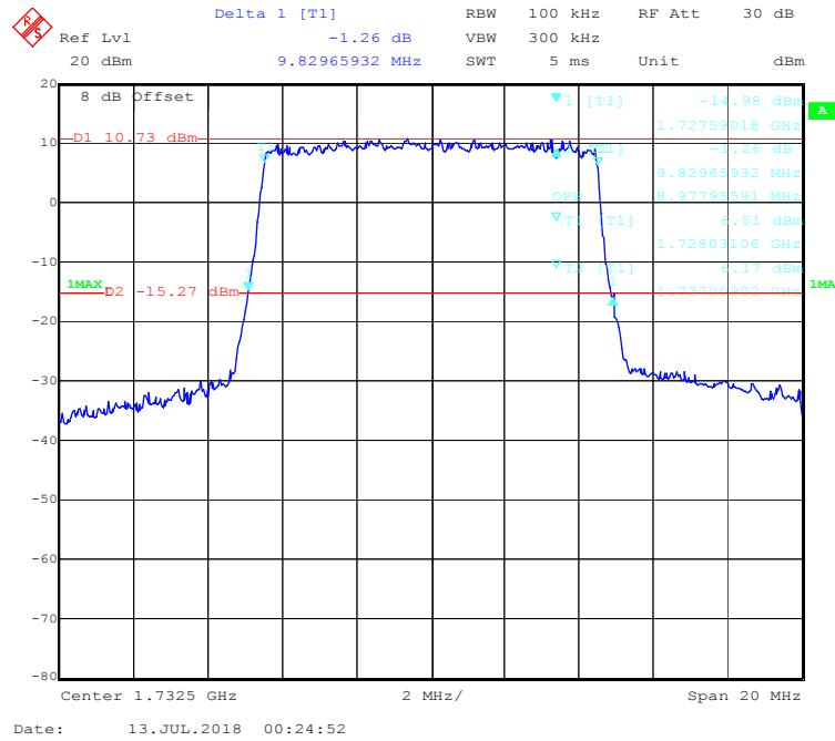
**QPSK (15.0 MHz) - 99% Occupied & 26 dB Emissions Bandwidth, Middle channel**
