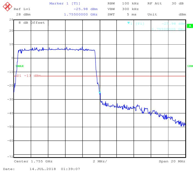
**QPSK (15.0 MHz, FULL RB) - Left Band Edge**
