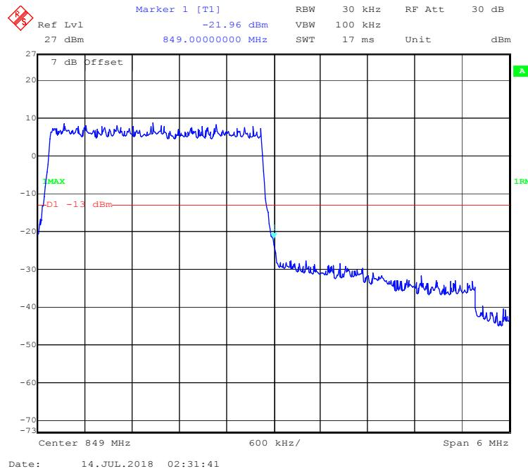
**16-QAM (5.0 MHz, FULL RB) - Left Band Edge**
