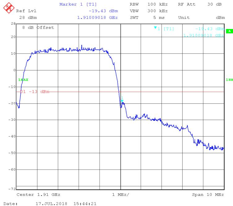
**LTE Band 2:****QPSK (1.4 MHz, FULL RB) - Left Band Edge**
