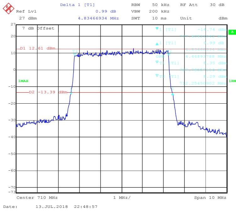
**16-QAM (10.0 MHz) - 99% Occupied & 26 dB Emissions Bandwidth, Middle channel**
