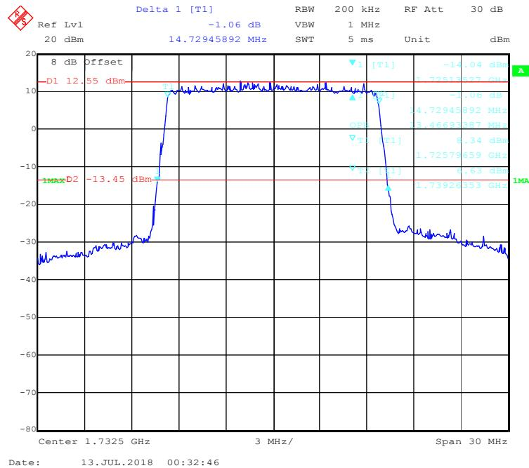
**16-QAM (20.0 MHz) - 99% Occupied & 26 dB Emissions Bandwidth, Middle channel**
