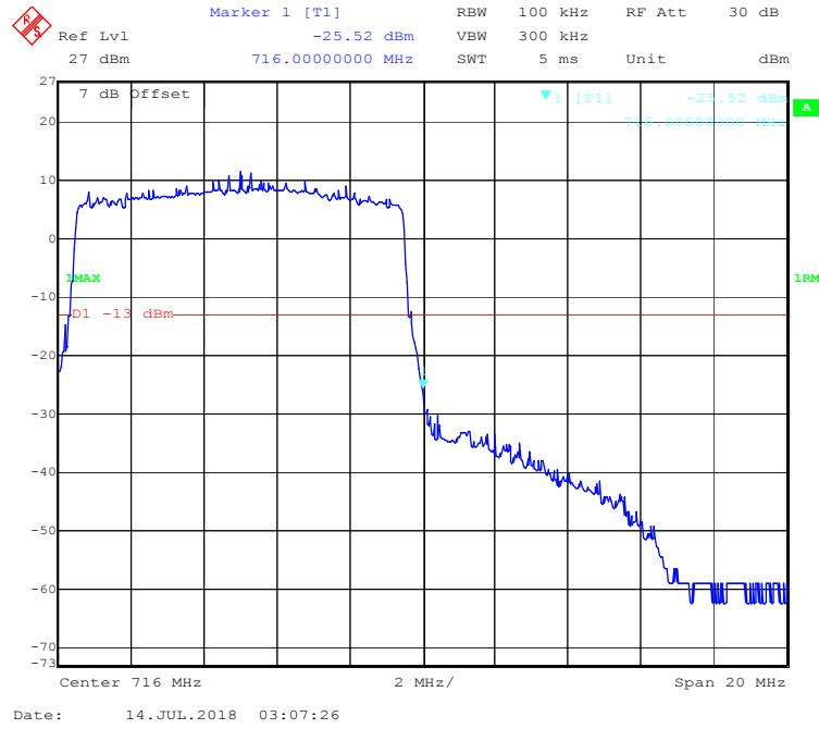
**16-QAM (1.4 MHz, FULL RB) - Left Band Edge**
