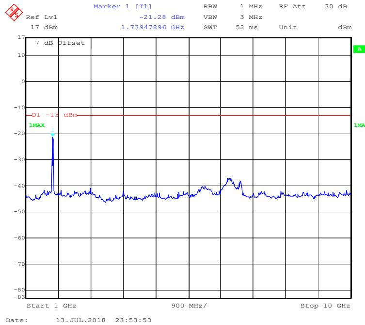
**LTE Band 12:****30 MHz - 1 GHz (1.4 MHz, Middle Channel)**
