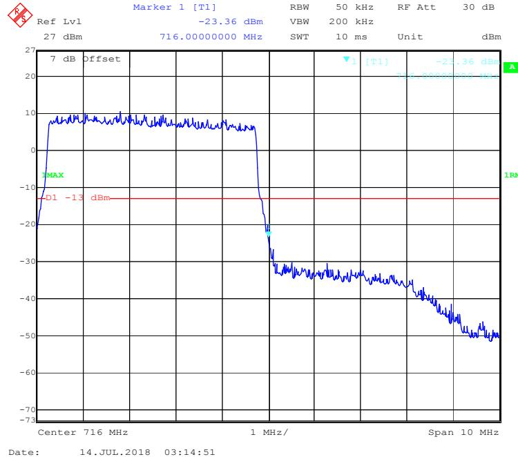
**QPSK (10.0 MHz, FULL RB) - Left Band Edge**
