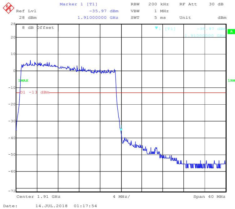
**LTE Band 4:****QPSK (1.4 MHz, FULL RB) - Left Band Edge**
