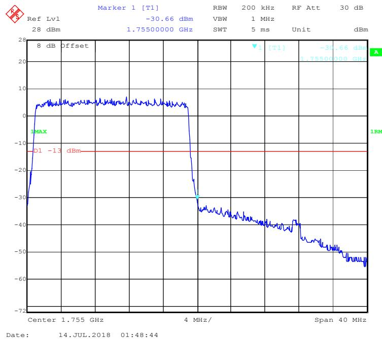
**16-QAM (1.4 MHz, FULL RB) - Left Band Edge**
