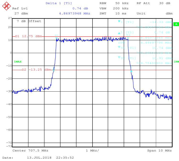
**16-QAM (10.0 MHz) - 99% Occupied & 26 dB Emissions Bandwidth, Middle channel**
