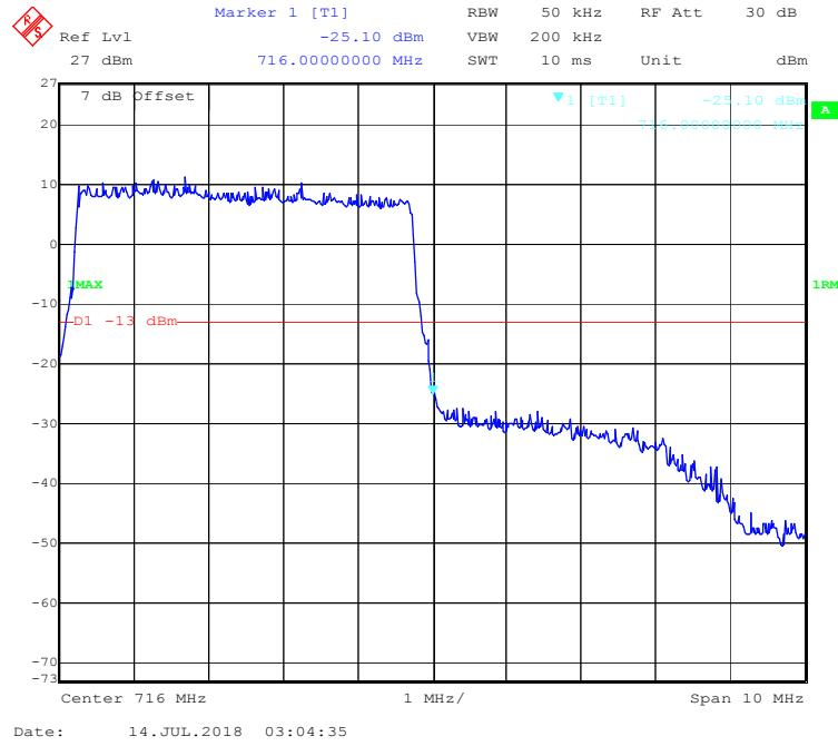
**16-QAM (10.0 MHz, FULL RB) - Left Band Edge**
