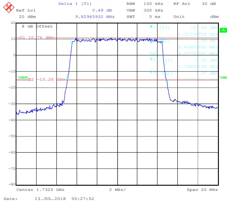
**16-QAM (15.0 MHz) - 99% Occupied & 26 dB Emissions Bandwidth, Middle channel**
