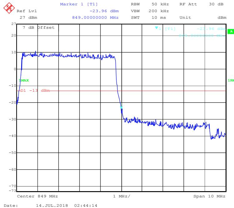
**16-QAM (10.0 MHz, FULL RB) - Left Band Edge**
