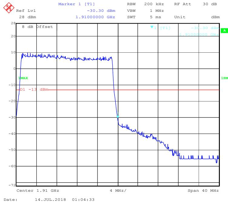
**16-QAM (1.4 MHz, FULL RB) - Left Band Edge**
