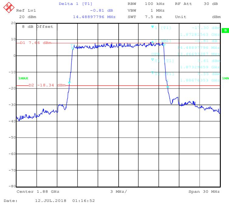
**QPSK (20.0 MHz) - 99% Occupied & 26 dB Emissions Bandwidth, Middle channel**
