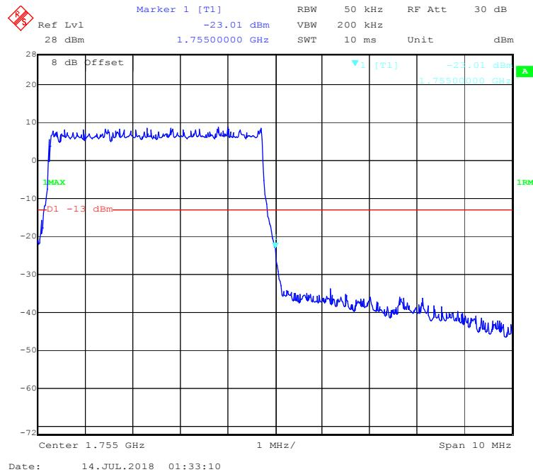
**QPSK (10.0 MHz, FULL RB) - Left Band Edge**
