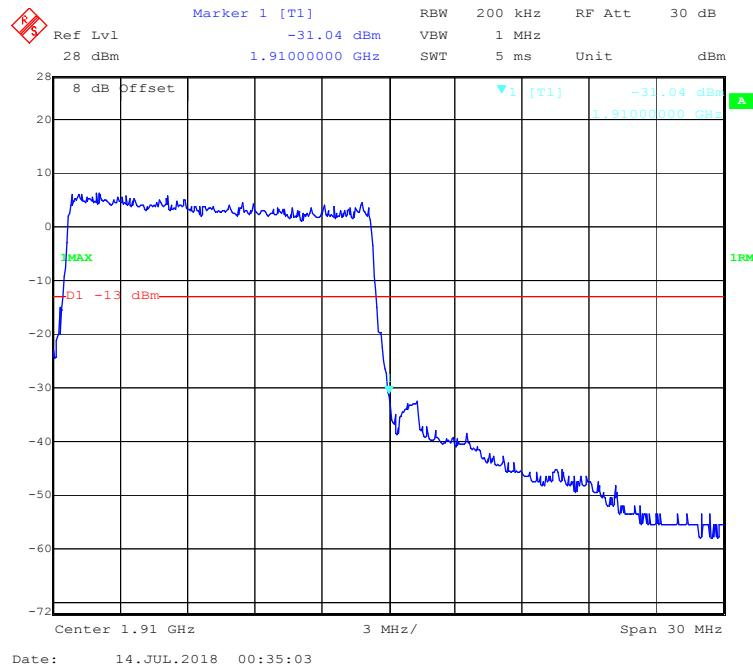
**QPSK (20.0 MHz, FULL RB) - Left Band Edge**
