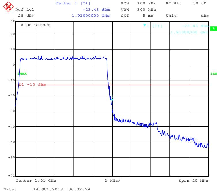
**QPSK (15.0 MHz, FULL RB) - Left Band Edge**
