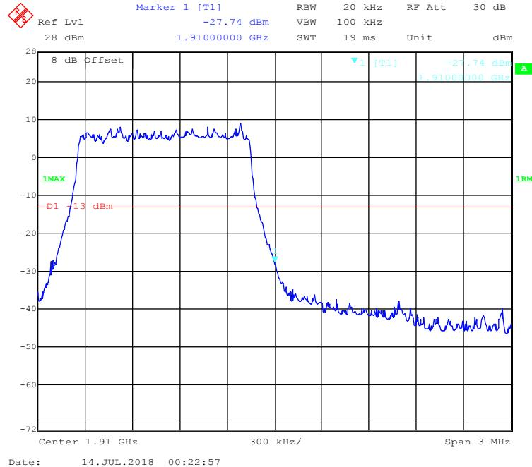
**QPSK (3.0 MHz, FULL RB) - Left Band Edge**
