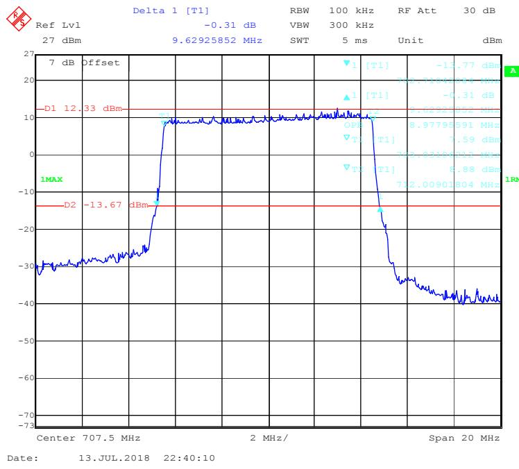
**16-QAM (1.4 MHz) - 99% Occupied & 26 dB Emissions Bandwidth, Middle channel**
