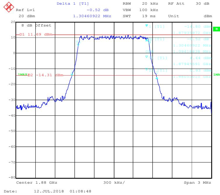
**QPSK (3.0 MHz) - 99% Occupied & 26 dB Emissions Bandwidth, Middle channel**
