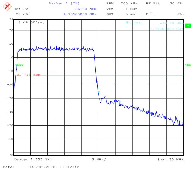
**QPSK (20.0 MHz, FULL RB) - Left Band Edge**
