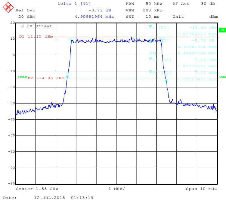
**QPSK (10.0MHz) - 99% Occupied & 26 dB Emissions Bandwidth, Middle channel**
