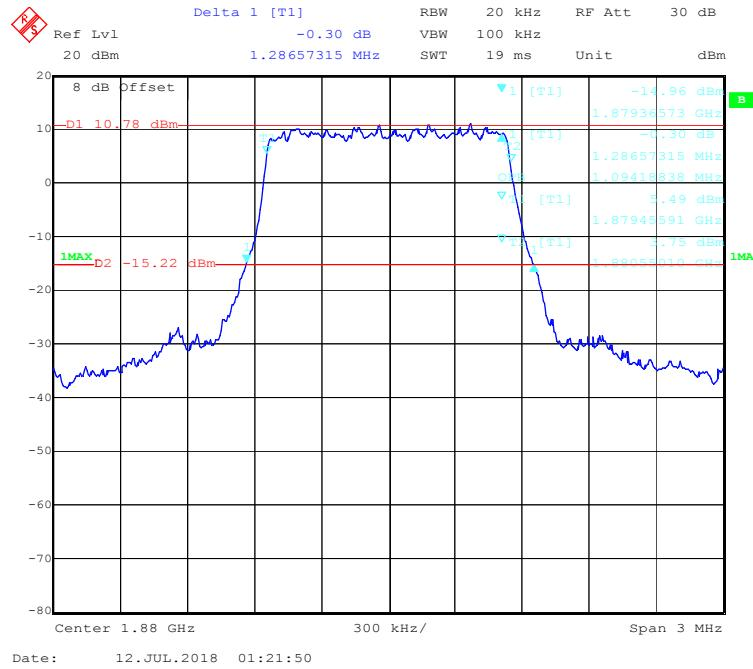
**16-QAM (3.0 MHz) - 99% Occupied & 26 dB Emissions Bandwidth, Middle channel**
