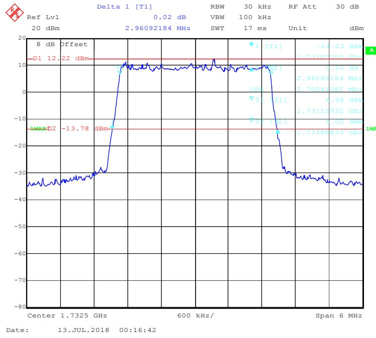
**QPSK (5.0MHz) - 99% Occupied & 26 dB Emissions Bandwidth, Middle channel**
