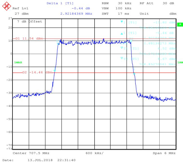
**QPSK (5.0 MHz) - 99% Occupied & 26 dB Emissions Bandwidth, Middle channel**
