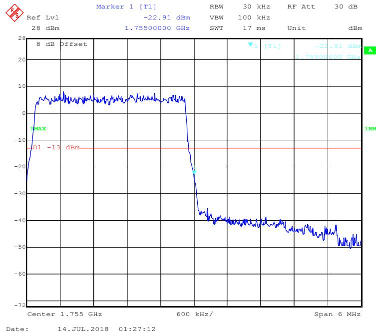
**QPSK (5.0 MHz, FULL RB) - Left Band Edge**
