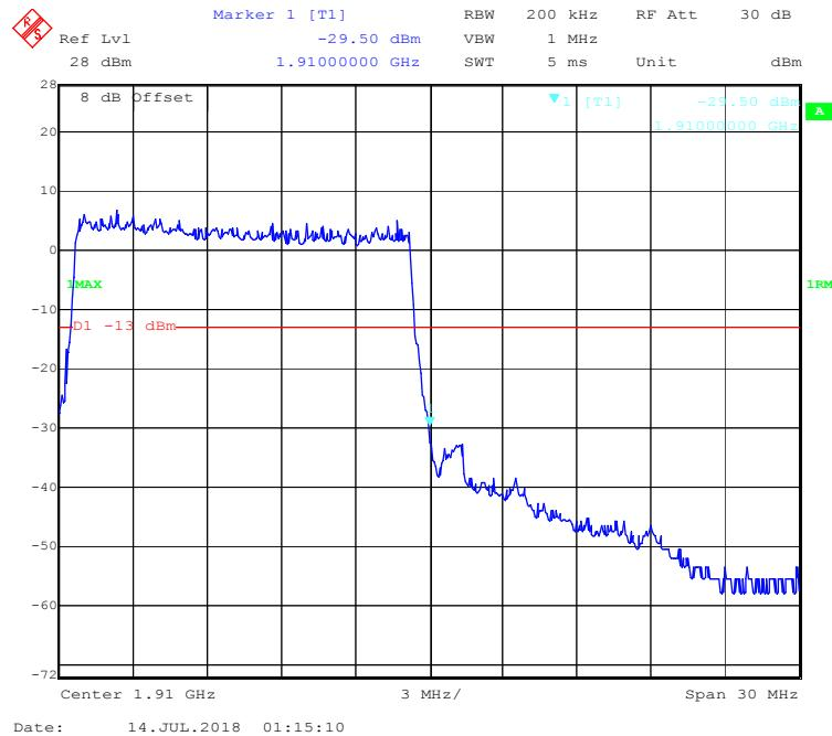
**16-QAM (20.0 MHz, FULL RB) - Left Band Edge**
