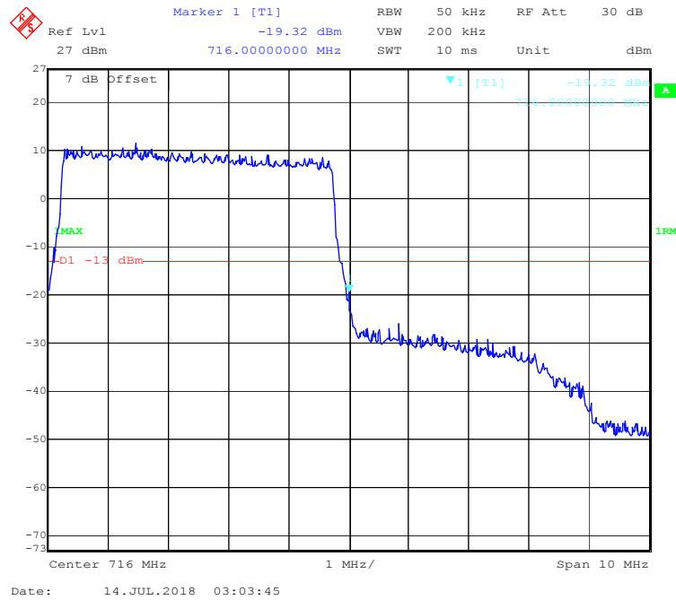
**QPSK (10.0 MHz, FULL RB) - Left Band Edge**
