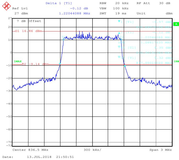
**QPSK (3.0 MHz) - 99% Occupied & 26 dB Emissions Bandwidth, Middle channel**
