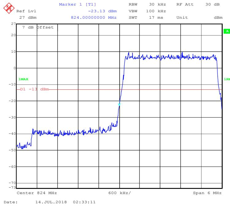
**QPSK (3.0 MHz, FULL RB) - Right Band Edge**
