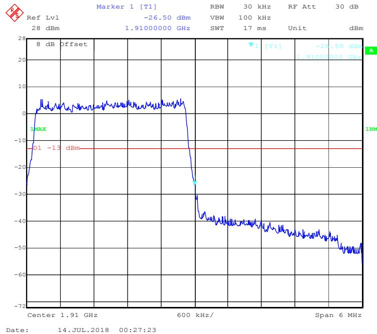
**QPSK (5.0 MHz, FULL RB) - Left Band Edge**
