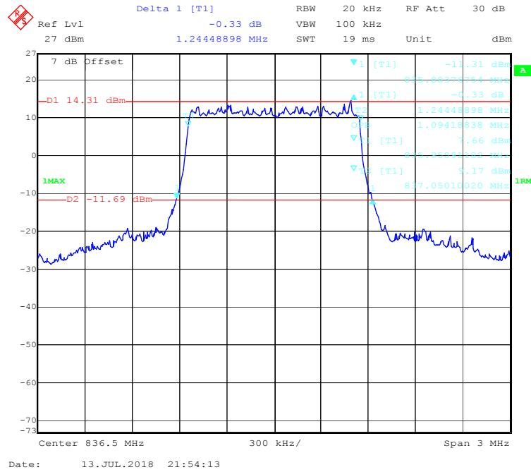
**16-QAM (3.0 MHz) - 99% Occupied & 26 dB Emissions Bandwidth, Middle channel**
