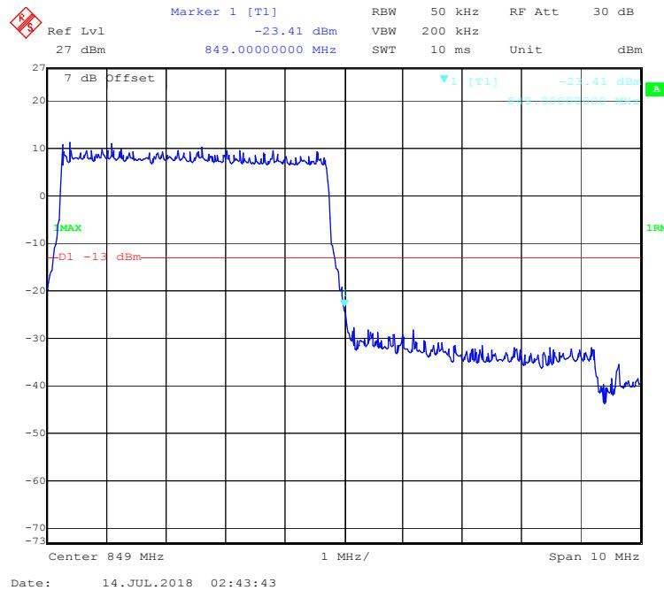
**QPSK (10.0 MHz, FULL RB) - Left Band Edge**
