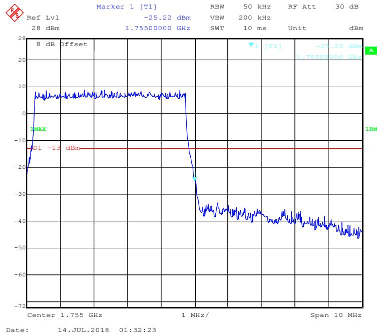
**16-QAM (10.0 MHz, FULL RB) - Left Band Edge**
