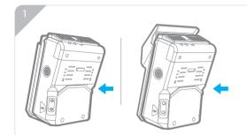
With the Mount Plate/the Wedge Mount Plate attached to the windshield and the power cord connected to the Al Recorder, position the Al Recorder on the upside of the Mount Plate/the Wedge Mount Plate. Next, ensure the Mount Plate/the Wedge Mount Plate locking tabs are aligned with their fittings on the recorder.
