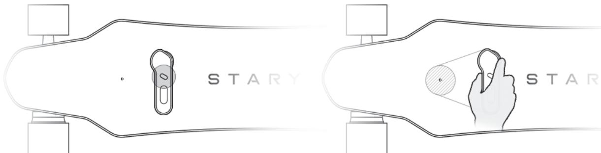
Put the remote (with screen side up) in the induction zone tagged on the griptape. The remote will vibrate to indicate that the skateboard has been switched on.
