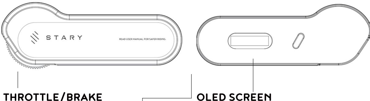
Large thumb-wheel with wider range and more accurate speed control
