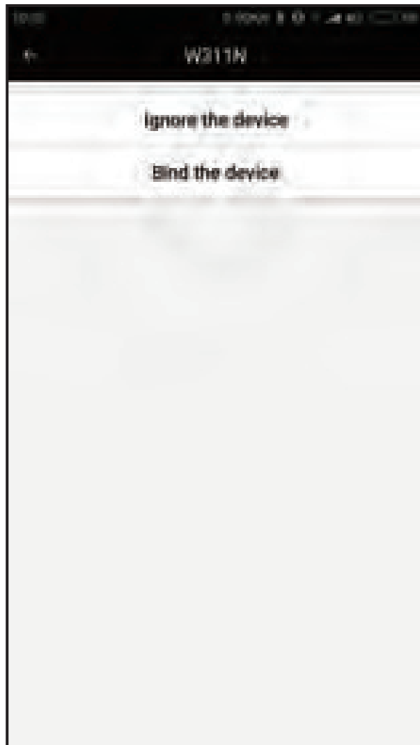
Press W311N and Bind the device
