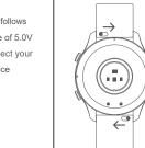
Slide the spring pin and hold it while pulling away from the watch to remove the current wristband. To attach a new band, slide the spring pin across and slot the new band. When both sides of the band are positioned correctly, release the spring pin.
