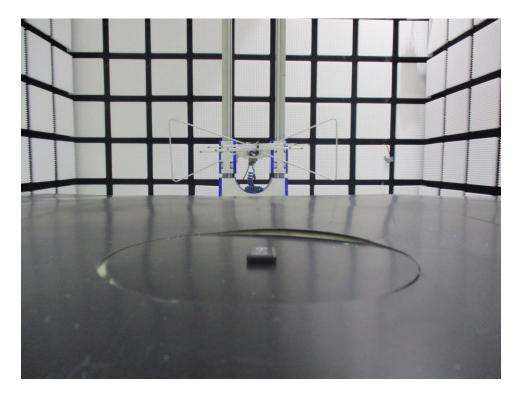
Radiated Emission test above 1GHz
