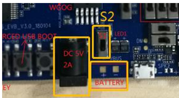
Figure 3-1: L710 development board power in Status (orange Power LED Light up)
