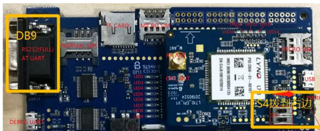
Figure5-1: L710 RS232 (DB9) Port
