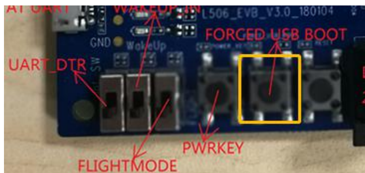
Figure 4-2: forced usb download key
