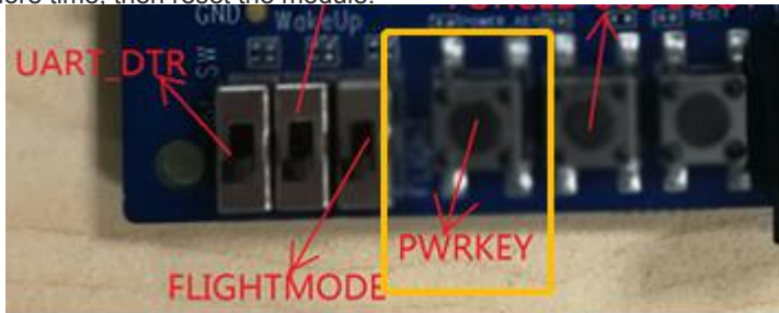
Figure 4-1: Power on/off reset key
